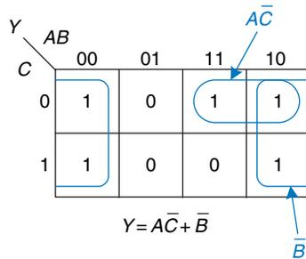
**Figure 2.46** Solution for Example 2.9
