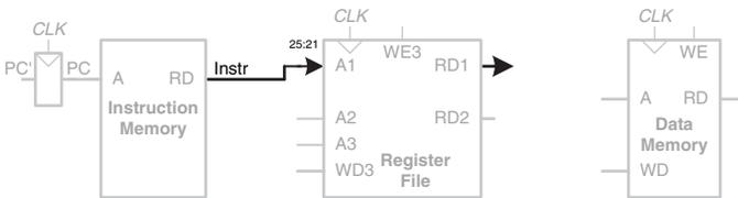
**Figure 7.3** Read source operand from register file
