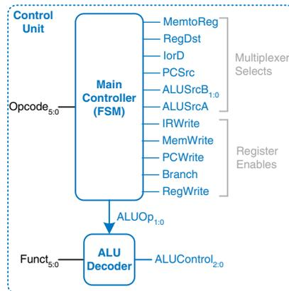
Figure 7.28 Control unit internal structure
