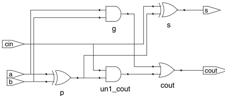
**Figure 4.8** fulladder synthesized circuit
