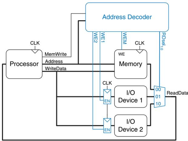
**Figure 8.28** Support hardware for memory-mapped I/O
