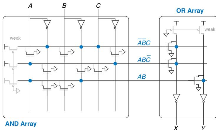
output HIGH for each wordline without a pull-down transistor. For example, when  $AB = 11$ , the 11 wordline is HIGH and transistors on X and Z turn on and pull those outputs LOW. The Y output has no transistor connecting to the 11 wordline, so Y is pulled HIGH by the weak pull-up.
