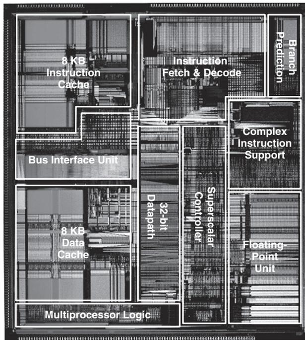
**Figure 7.77** Pentium III microprocessor chip
