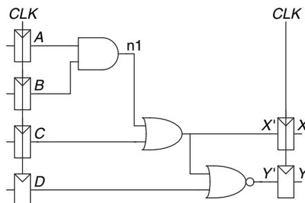
**Figure 3.42** Sample circuit for timing analysis
