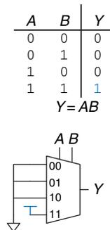
**Figure 2.59** 4:1 multiplexer implementation of two-input AND function
