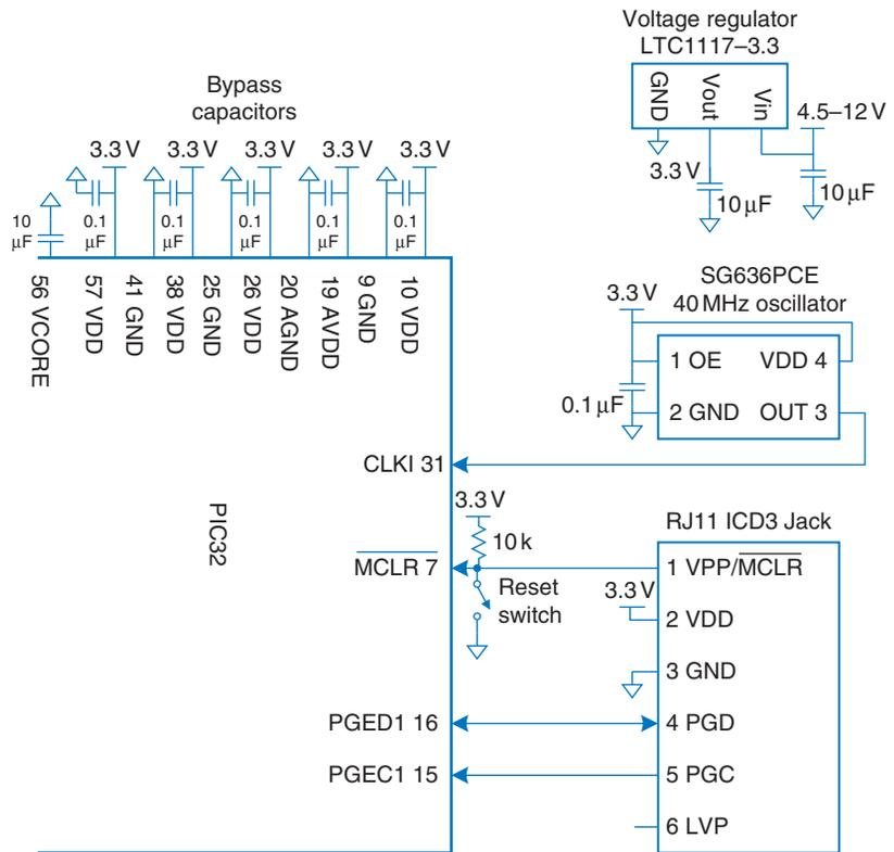
The peripheral bus clock PBCLK can be configured to operate at the same speed as the main system clock, or at half, a quarter, or an eighth of the speed. Early PIC32 microcontrollers were limited to a maximum of half-speed operation because some peripherals were too slow, but most current products can run at full speed. If you change the PBCLK speed, you'll need to adjust parts of the sample code in this section such as the number of PBCLK ticks to measure a certain amount of time.
