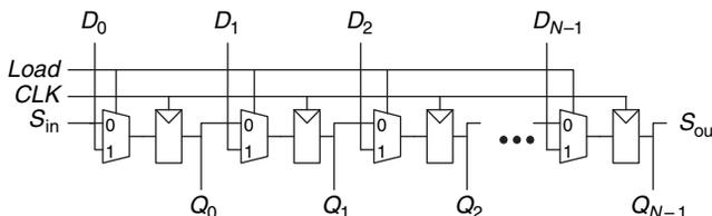
Figure 5.35 Shift register with parallel load
