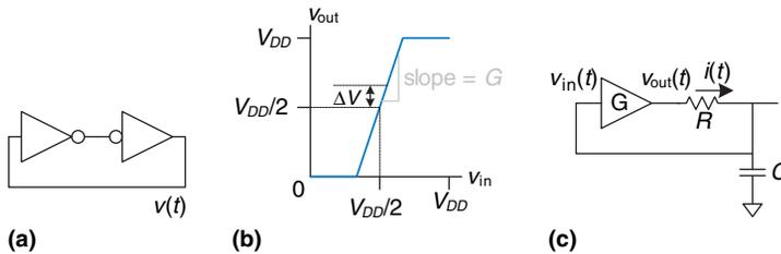
Figure 3.55 Circuit model of bistable device
