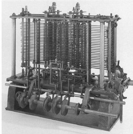
of the Analytical Engine, in which each row processes one digit. Babbage chose 25 rows of gears, so the machine has 25-digit precision.
