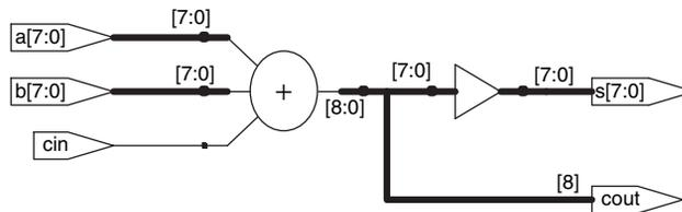
Figure 5.8 Synthesized adder
