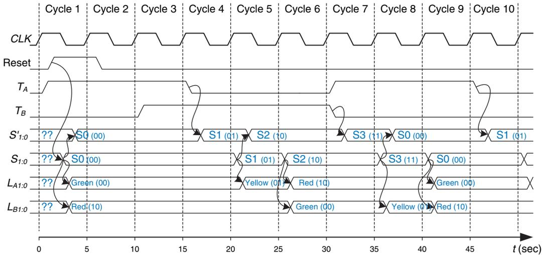
Figure 3.27 Timing diagram for traffic light controller
