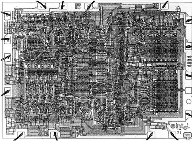
**Figure 7.73** 4004 microprocessor chip
