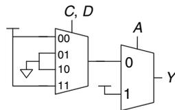
Figure 2.87 Multiplexer circuit
