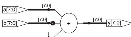
Figure 5.10 Synthesized subtractor
