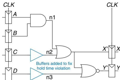
Figure 3.44 Corrected circuit to fix hold time problem
