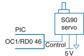
**Figure 8.64** Servo motor control
