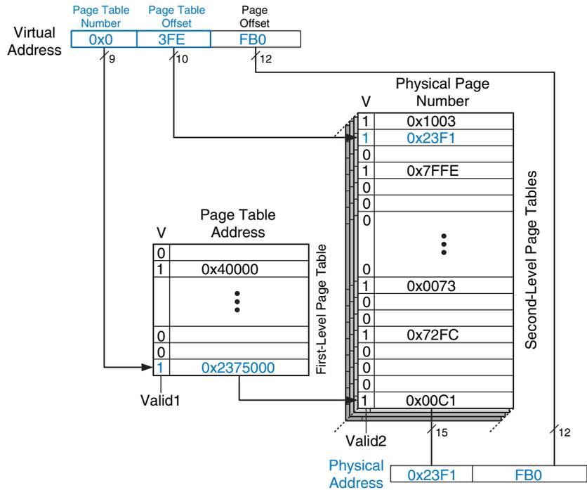
Figure 8.27 Address translation using a two-level page table
