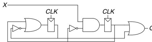
**Exercise 3.32** Repeat Exercise 3.31 for the FSM shown in Figure 3.73. Recall that the  $s$  and  $r$  register inputs indicate set and reset, respectively.
