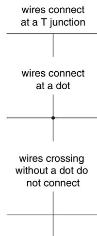
**Figure 2.24** Wire connections
