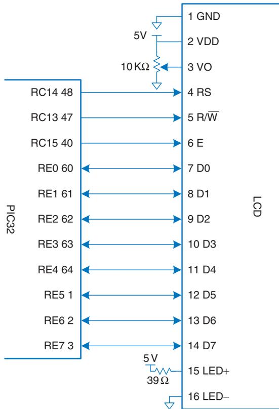
**Figure 8.50** Parallel LCD interface
