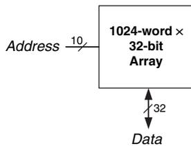
**Figure 5.40** 32 Kb array: depth =  $2^{10} = 1024$  words, width = 32 bits
