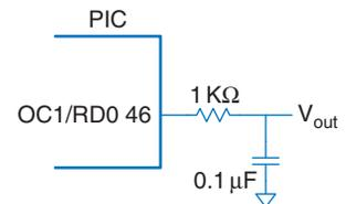
**Figure 8.48** Analog output using PWM and low-pass filter
