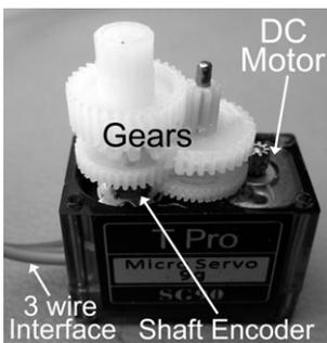
**Figure 8.62** SG90 servo motor
