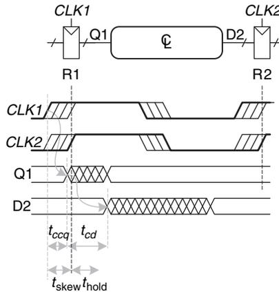
**Figure 3.49** Hold time constraint with clock skew
