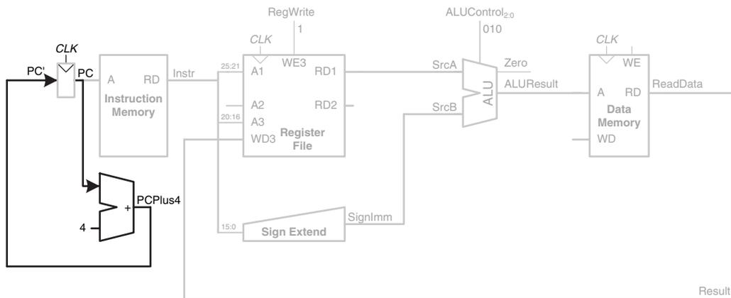
Figure 7.7 Determine address of next instruction for PC
