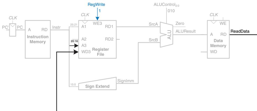
Figure 7.6 Write data back to register file
