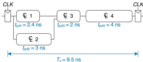
Figure 3.58 Circuit with no pipelining
