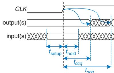
**Figure 3.37** Timing specification for synchronous sequential circuit
