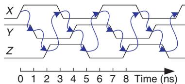
Figure 3.17 Ring oscillator waveforms
