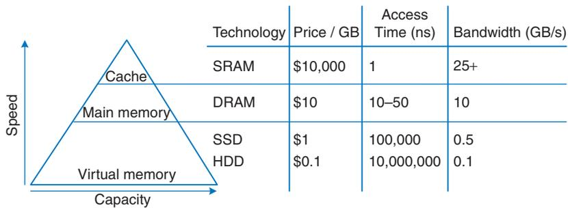
**Figure 8.4** Memory hierarchy components, with typical characteristics in 2012
