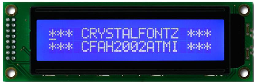
**Figure 8.49** Crystallfontz CFAH2002A-TMI 20  $\times$  2 character LCD
