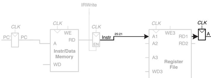
**Figure 7.18** Read source operand from register file
