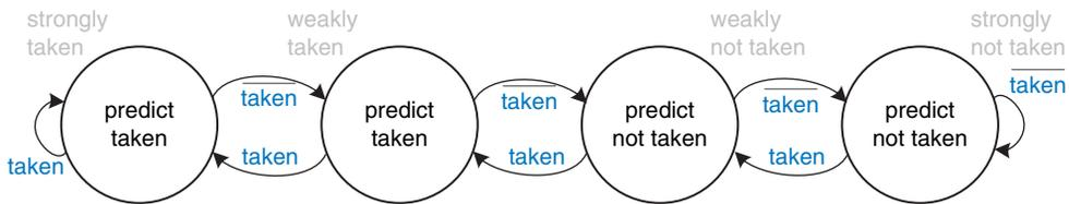
**Figure 7.66** 2-bit branch predictor state transition diagram
