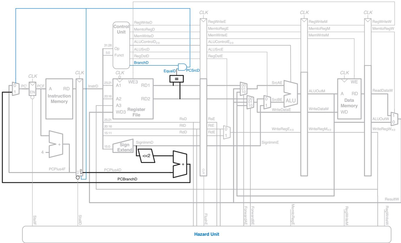
**Figure 7.56** Pipelined processor handling branch control hazard
