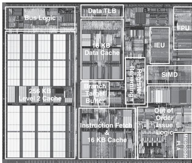
The floating-point datapath is called the Floating Point Unit (FPU). The processor also has a SIMD unit to perform packed operations on short integer and floating-point data. A larger portion of the chip is dedicated to issuing instructions out-of-order than to actually executing the instructions. The instruction and data caches have grown to 16 KB each. The Pentium III also has a larger but slower 256-KB second-level cache on the same chip.
