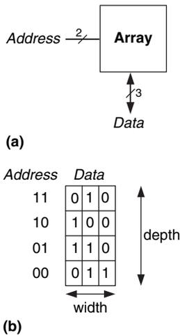
**Figure 5.39**  $4 \times 3$  memory array: (a) symbol, (b) function
