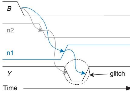
As long as we wait for the propagation delay to elapse before we depend on the output, glitches are not a problem, because the output eventually settles to the right answer.
