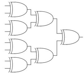
**Figure 2.32** Eight-input XOR using seven two-input XORs
