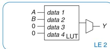
**Figure 5.59** LE configuration for two functions of up to four inputs each
