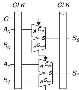
Figure 3.75 2-bit adder schematic
