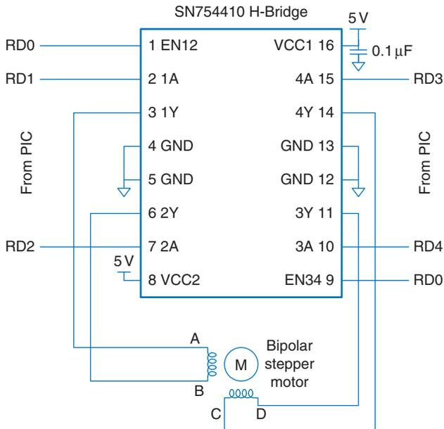
**Figure 8.69** Bipolar stepper motor direct drive with H-bridge
