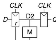
**Figure 3.76** “New and improved” synchronizer
