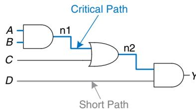
**Figure 2.68** Short path and critical path
