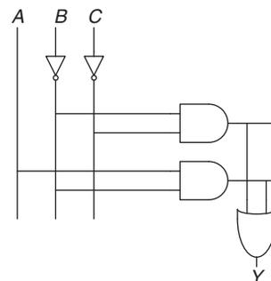
**Figure 2.25** Schematic of  $Y = \bar{B} \bar{C} + A \bar{B}$
