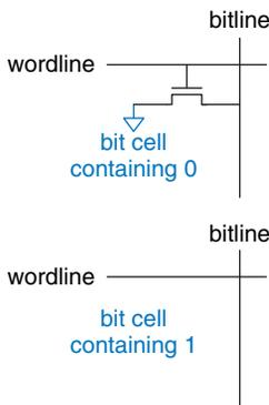
**Figure 5.48** ROM bit cells containing 0 and 1
