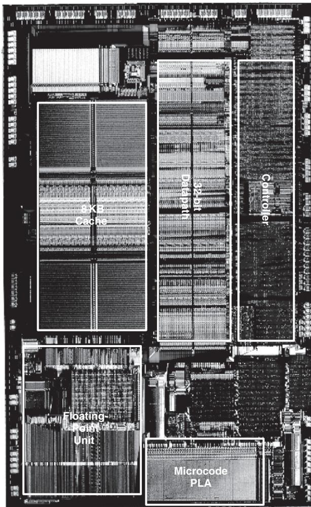
**Figure 7.75** 80486 microprocessor chip
