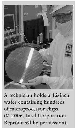
A technician holds a 12-inch wafer containing hundreds of microprocessor chips (© 2006, Intel Corporation. Reproduced by permission).
