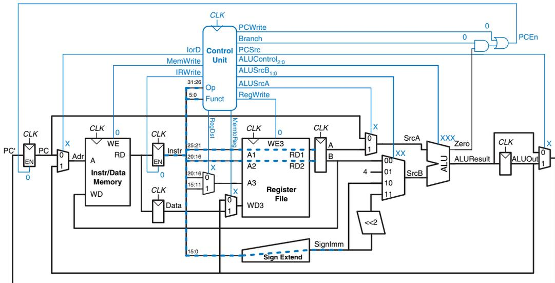
Figure 7.32 Data flow during the decode step
