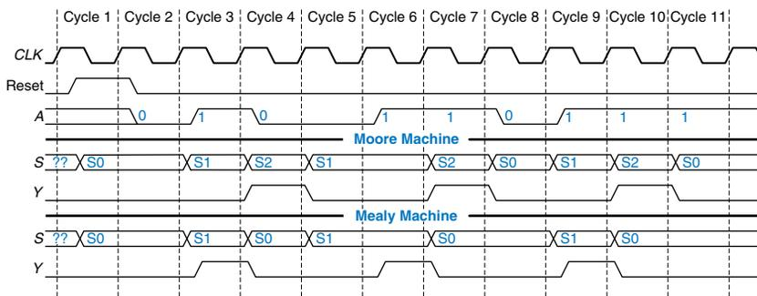
**Figure 3.32** Timing diagrams for Moore and Mealy machines
