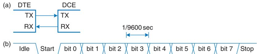
**Figure 8.40** Asynchronous serial link
