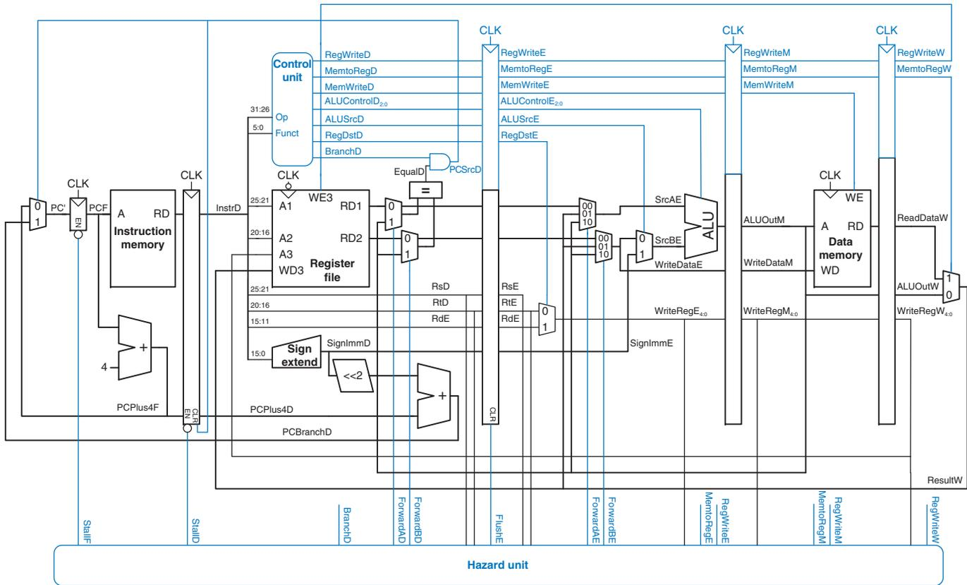
Figure 7.58 Pipelined processor with full hazard handling
