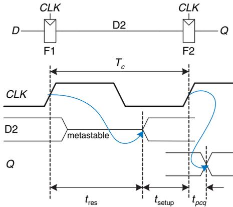
Figure 3.53 Simple synchronizer
