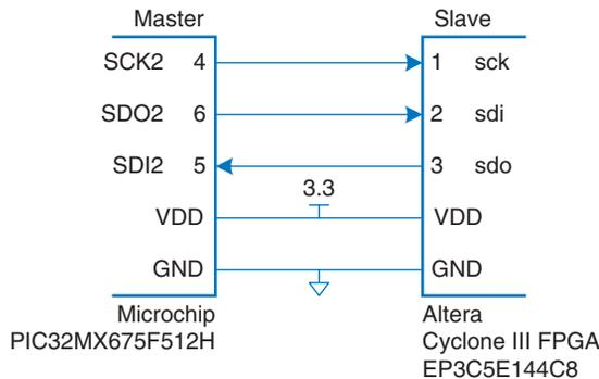
**Figure 8.37** SPI connection between PIC32 and FPGA
