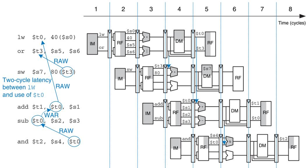
Figure 7.70 Out-of-order execution of a program with dependencies
