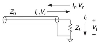
**Figure A.35** Transmission line showing incoming, reflected, and load voltages and currents
