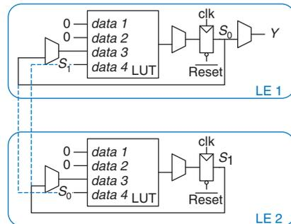
using the multiplexer on *data 3* and routing channels between LEs, as indicated by the dashed blue lines. In general, another LE might be necessary to compute the output *Y*. However, in this case  $Y = S_0$ , so *Y* can come from LE 1. Hence, the entire FSM fits in two LEs. In general, an FSM requires at least one LE for each bit of state, and it may require more LEs for the output or next state logic if they are too complex to fit in a single LUT.
