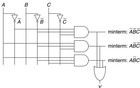
**Figure 2.23** Schematic of  $Y = \bar{A} \bar{B} \bar{C} + A \bar{B} \bar{C} + A B \bar{C}$
