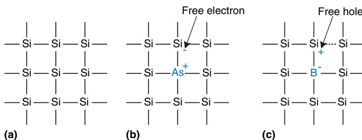
**Figure 1.26** Silicon lattice and dopant atoms
