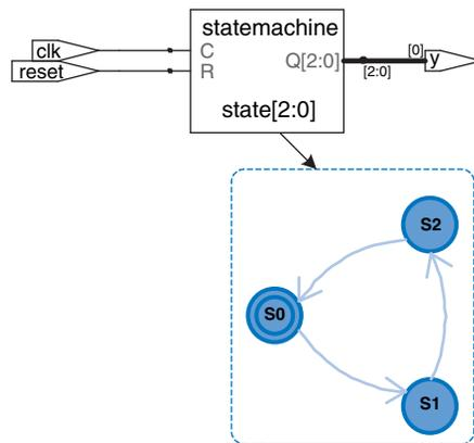
**Figure 4.25** divideby3fsm synthesized circuit
