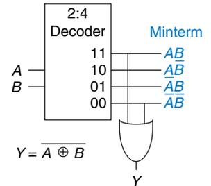
Figure 2.65 Logic function using decoder
