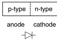
**Figure 1.27** The p-n junction diode structure and symbol
