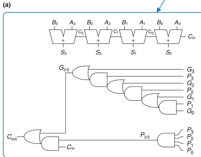
**Figure 5.6** (a) 32-bit carry-lookahead adder (CLA), (b) 4-bit CLA block
