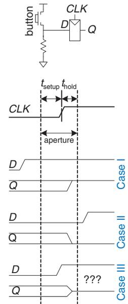
Figure 3.50 Input changing before, after, or during aperture
