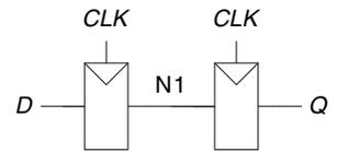
Figure 4.17 Synchronizer circuit
