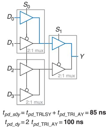
**Figure 2.74** 4:1 multiplexer propagation delays: hierarchical using 2:1 multiplexers
