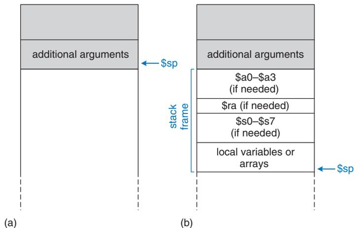
arguments, it finds them in the caller's stack frame. Accessing additional input arguments is the one exception in which a function can access stack data not in its own stack frame.
