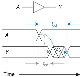
**Figure 2.67** Propagation and contamination delay
