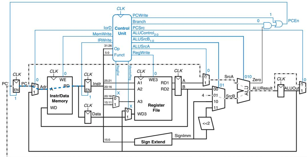
Figure 7.30 Data flow during the fetch step
