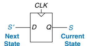
**Figure 3.20** Flip-flop current state and next state
