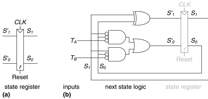
This schematic uses some AND gates with bubbles on the inputs. They might be constructed with AND gates and input inverters, with NOR gates and inverters for the non-bubbled inputs, or with some other combination of gates. The best choice depends on the particular implementation technology.
