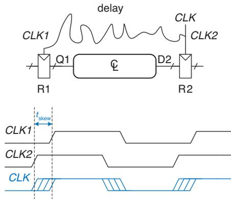
**Figure 3.46** Clock skew caused by wire delay
