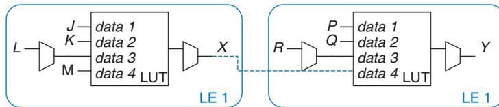
**Figure 5.61** LE configuration for FSM with two bits of state
