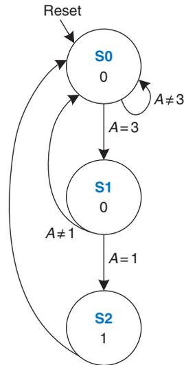
Alyssa writes down the state transition diagram shown in Figure 3.36 using Tables 3.21 and 3.22. By inspection, she can see that the finite state machine unlocks the door only after detecting an input value,  $A_{1:0}$ , of three followed by an input value of one. The door is then locked again. Alyssa tries this code on the door key pad and the door opens!
