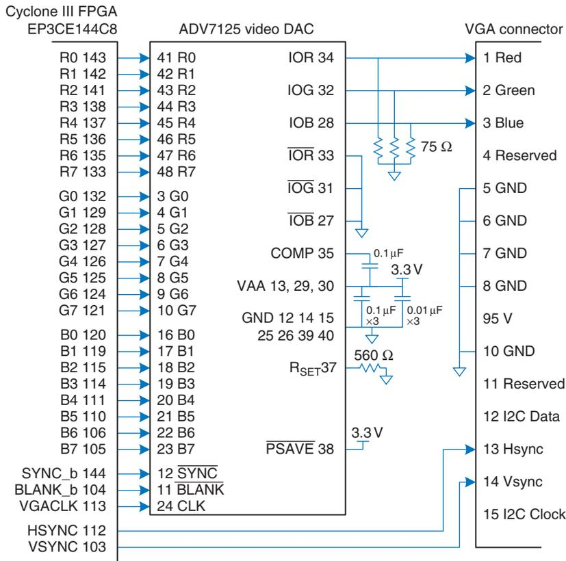
Figure 8.53 FPGA driving VGA cable through video DAC
