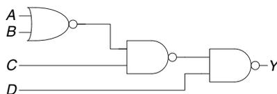
**Figure 2.33** Multilevel circuit using NANDs and NORs
