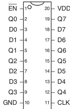
**74377 Register****8-bit Enableable Register**
