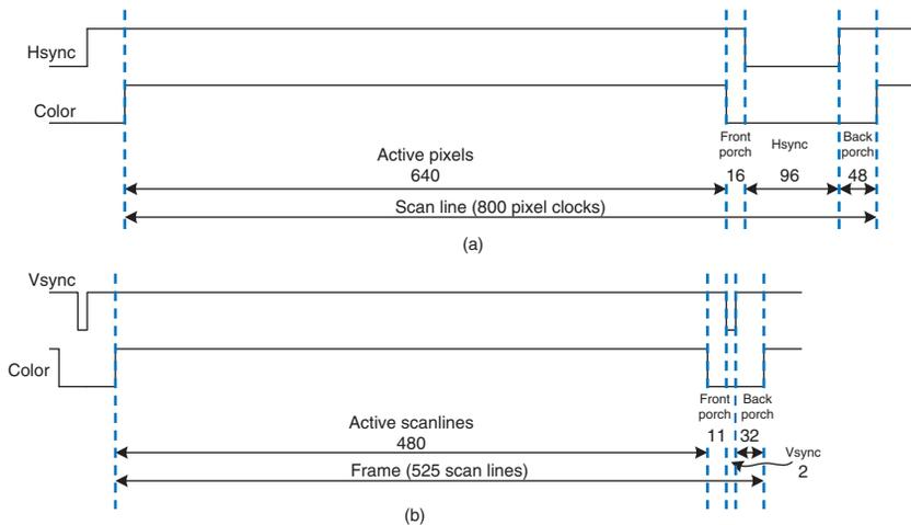
**Figure 8.51** VGA timing:
