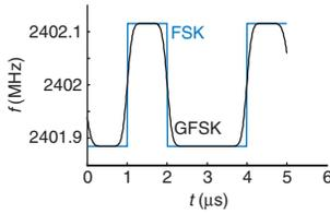
**Figure 8.55** FSK and GFSK waveforms
