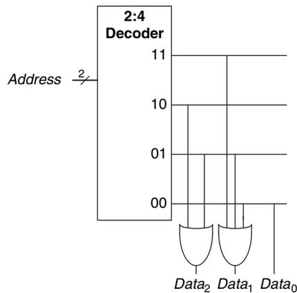
**Figure 5.50**  $4 \times 3$  ROM implementation using gates
