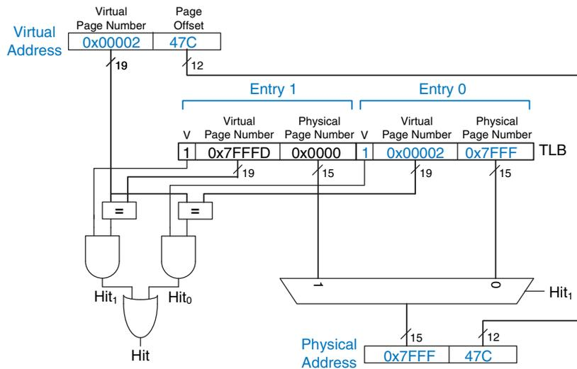
**Figure 8.25** Address translation using a two-entry TLB
