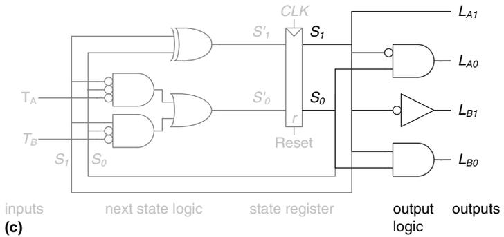
Figure 3.26 State machine circuit for traffic light controller
