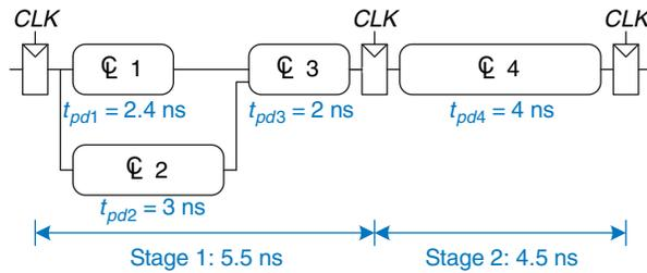
**Figure 3.60** Circuit with three-stage pipeline
