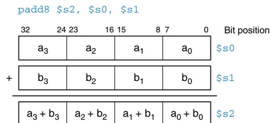
**Figure 7.72** Packed arithmetic: four simultaneous 8-bit additions
