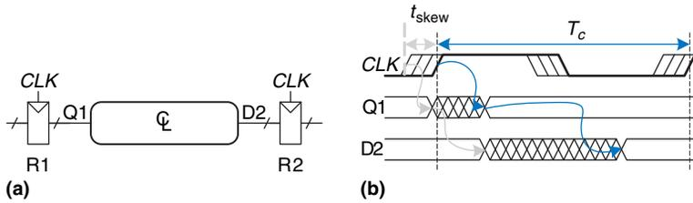
Figure 3.47 Timing diagram with clock skew
