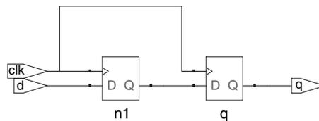
Figure 4.18 sync synthesized circuit
