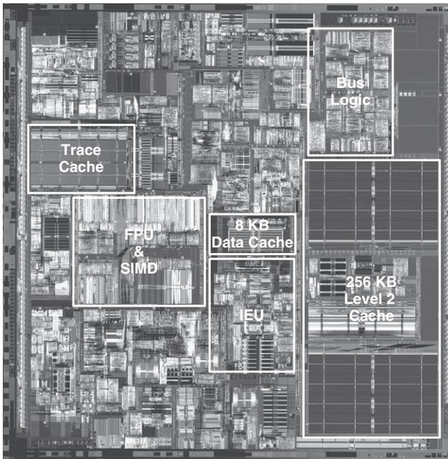
**Figure 7.78** Pentium 4 microprocessor chip
