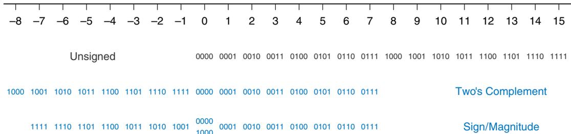
**Figure 1.11** Number line and 4-bit binary encodings
