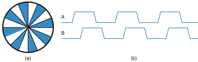
**Figure 8.61** Shaft encoder (a) disk, (b) quadrature outputs
