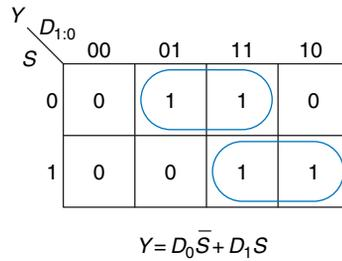
**Figure 2.55** 2:1 multiplexer implementation using two-level logic
