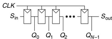
Figure 5.34 Shift register schematic
