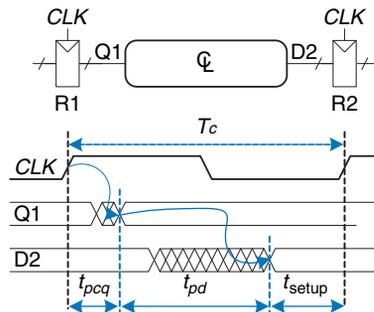
Figure 3.39 Maximum delay for setup time constraint
