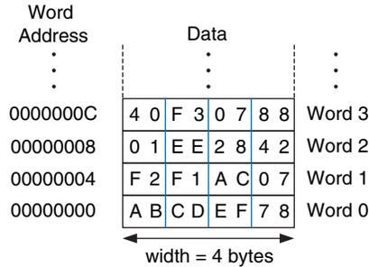
address ( $\$0 + 1$ ) = 1. After the load word instruction (`lw`) is executed, `$s3` holds the value `0xF2F1AC07`, which is the data value stored at memory address 1 in [Figure 6.1](#).
