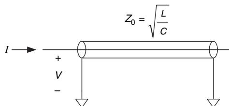
Figure A.15 Transmission line symbol
