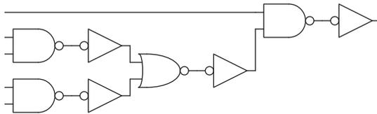
**Figure 2.37** Poor circuit using NANDs and NORs
