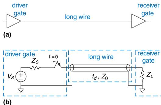
**Figure A.36** Digital system modeled with transmission line
