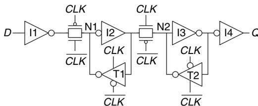
Figure 3.13 D flip-flop schematic
