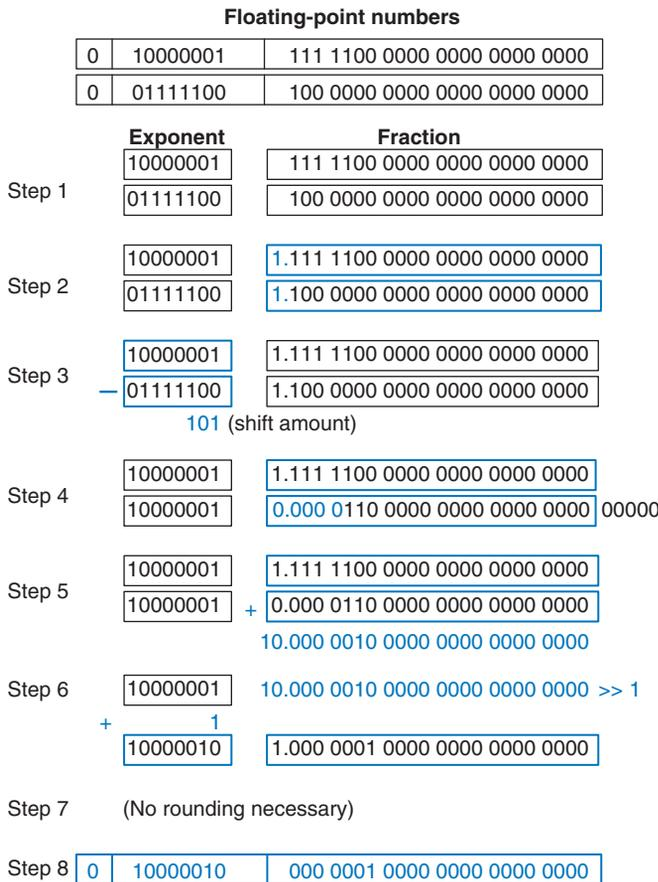
**Figure 5.29** Floating-point addition
