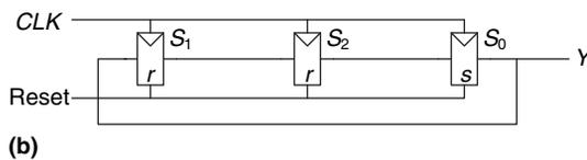
**Figure 3.29** Divide-by-3 circuits for (a) binary and (b) one-hot encodings
