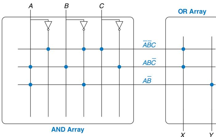
Figure 5.55  $3 \times 3 \times 2$ -bit PLA: dot notation
