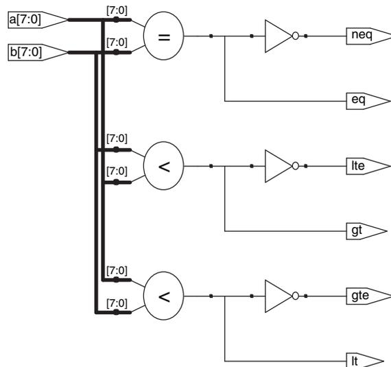
Figure 5.13 Synthesized comparators
