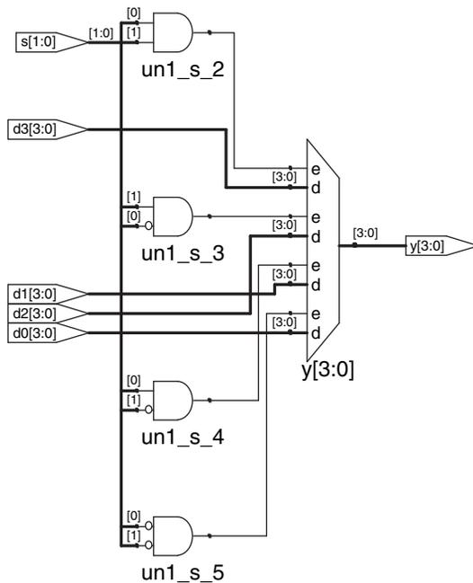
**Figure 4.7** mux4 synthesized circuit
