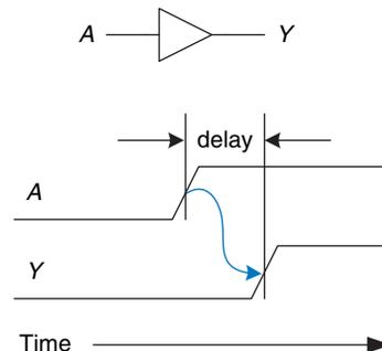
Figure 2.66 Circuit delay
