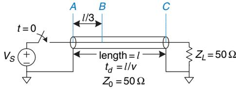
**Figure A.16** Transmission line with matched termination
