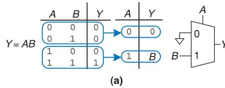
**Figure 2.60** Multiplexer logic using variable inputs
