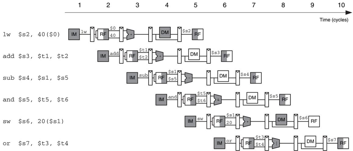
Figure 7.44 Abstract view of pipeline in operation
