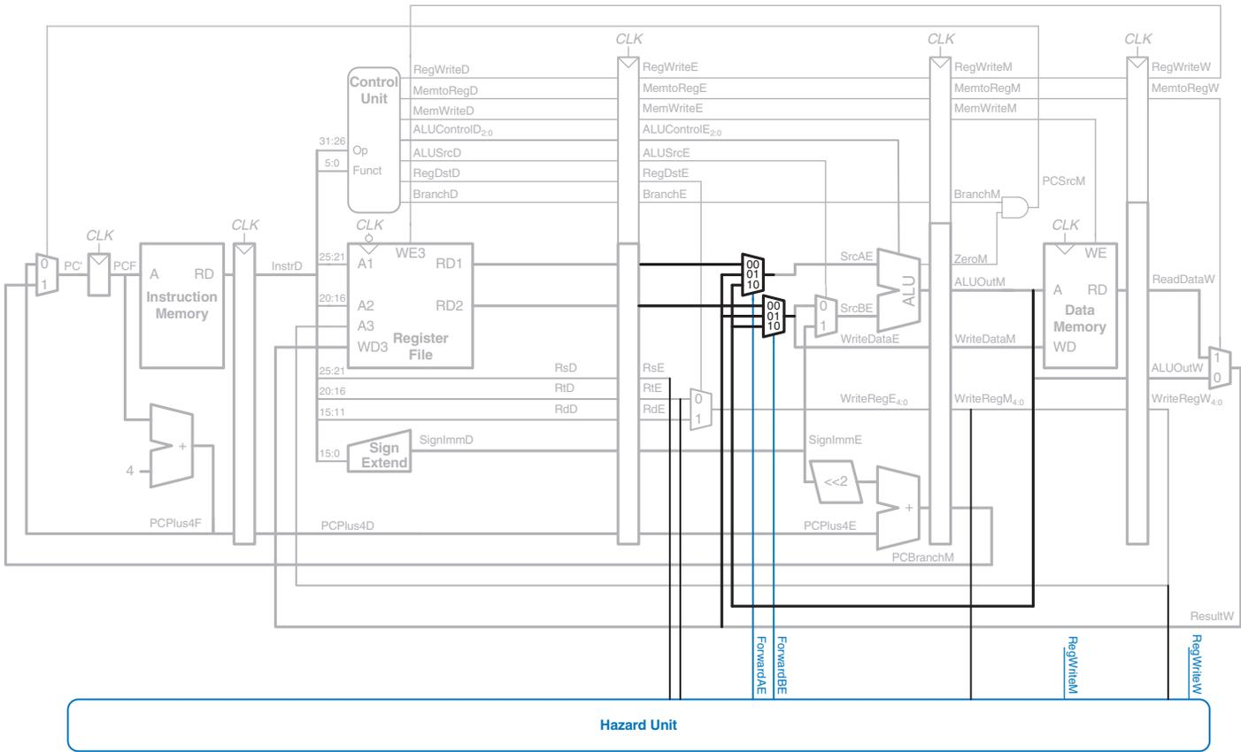
**Figure 7.50** Pipelined processor with forwarding to solve hazards
