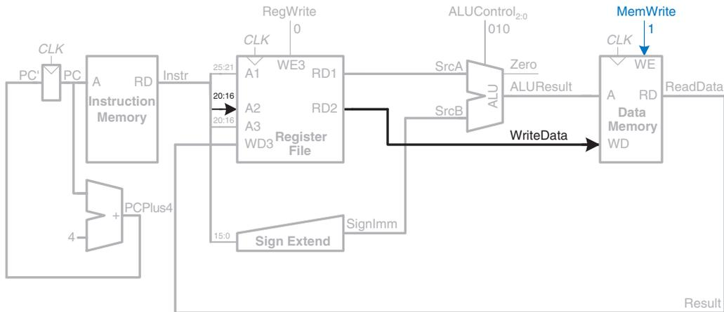
**Figure 7.8** Write data to memory for *sw* instruction
