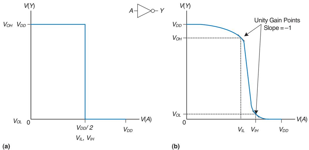
**Figure 1.25** DC transfer characteristics and logic levels
