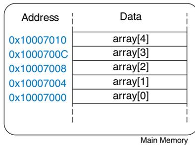
**Figure 6.20** Five-entry array with base address of 0x10007000
