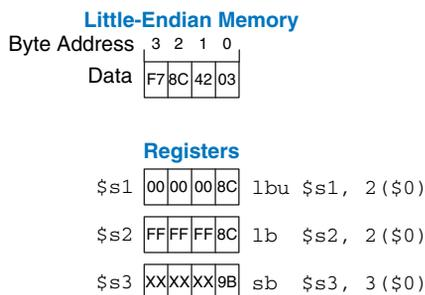
**Figure 6.22** Instructions for loading and storing bytes
