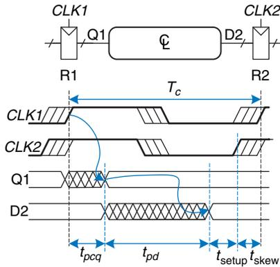
Figure 3.48 Setup time constraint with clock skew
