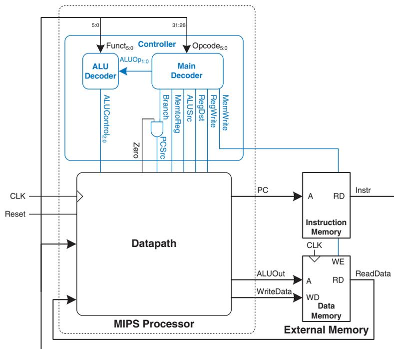
**Figure 7.59** MIPS single-cycle processor interfaced to external memory
