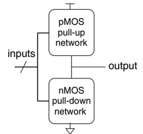
Figure 1.34 General form of an inverting logic gate
