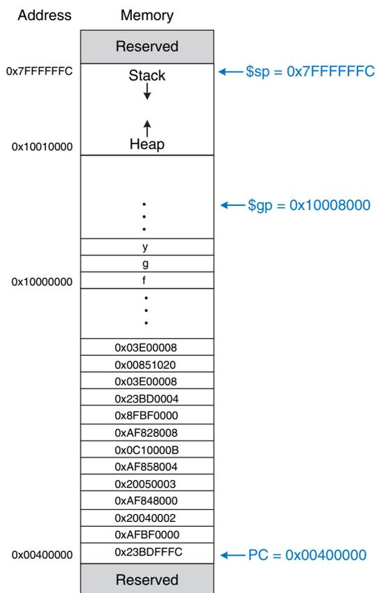
**Figure 6.34** Executable loaded in memory
