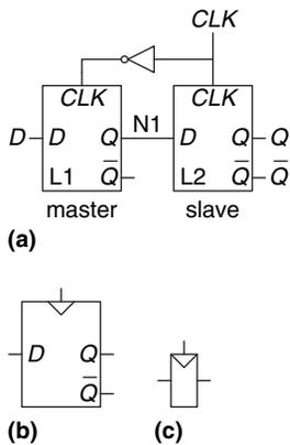
**Figure 3.8** D flip-flop:
