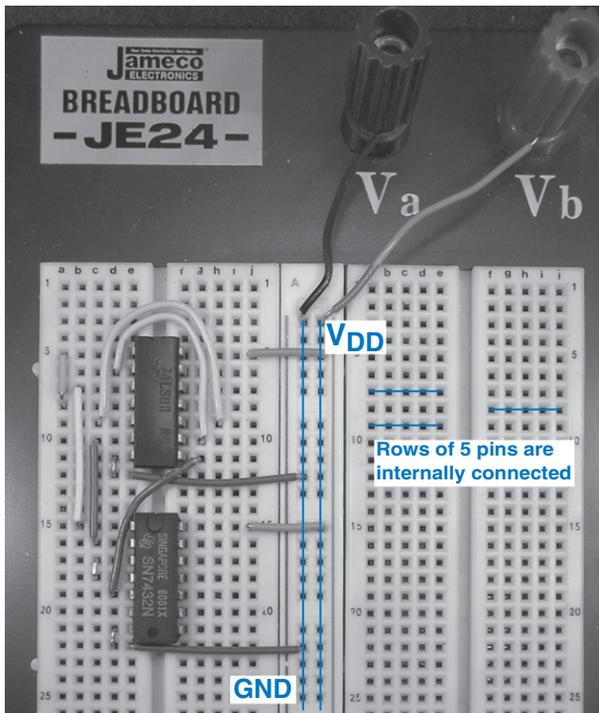
**Figure A.11** Majority circuit on breadboard
