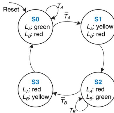
**Figure 3.25** State transition diagram
