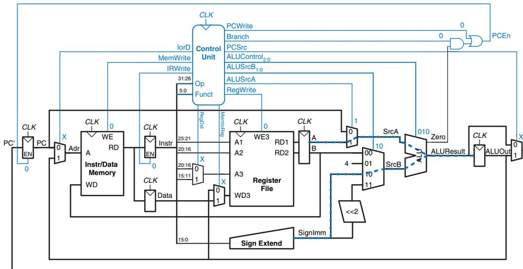
**Figure 7.34** Data flow during memory address computation
