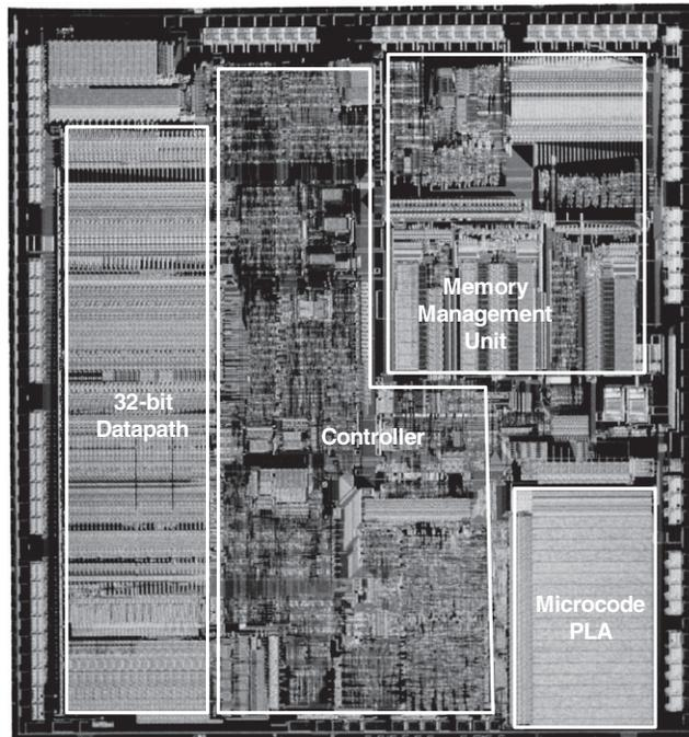
Figure 7.74 80386 microprocessor chip
