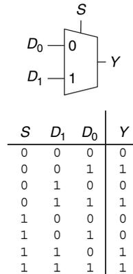
Figure 2.54 2:1 multiplexer symbol and truth table
