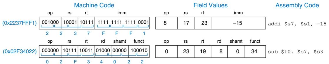
Figure 6.12 Machine code to assembly code translation
