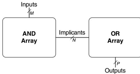
Figure 5.54  $M \times N \times P$ -bit PLA
