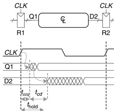
**Figure 3.40** Minimum delay for hold time constraint
