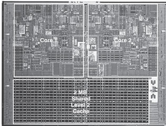
**Figure 7.79** Core Duo microprocessor chip
