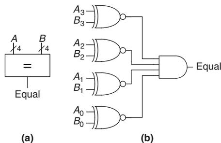
Figure 5.11 4-bit equality comparator: (a) symbol, (b) implementation
