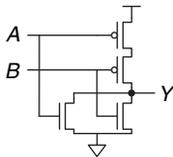
**Figure 1.36** Two-input NOR gate schematic
