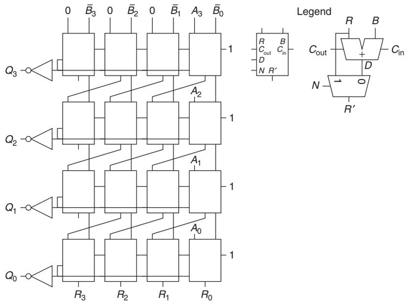
Figure 5.20 Array divider
