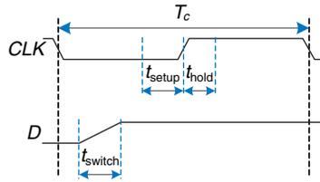
Figure 3.54 Input timing
