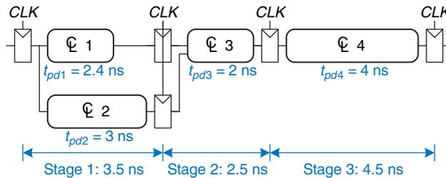
is two clock cycles, or 11 ns. The throughput is  $1/5.5 \text{ ns} = 182 \text{ MHz}$ . This example shows that, in a real circuit, pipelining with two stages almost doubles the throughput and slightly increases the latency. In comparison, ideal pipelining would exactly double the throughput at no penalty in latency. The discrepancy comes about because the circuit cannot be divided into two exactly equal halves and because the registers introduce more sequencing overhead.
