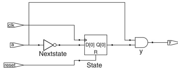
**Figure 4.27** patternMealy synthesized circuit**4.7 DATA TYPES\***
