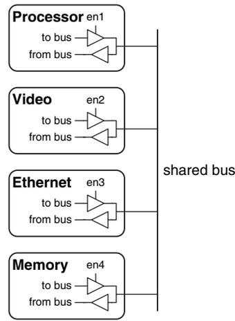
**Figure 2.42** Tristate bus connecting multiple chips
