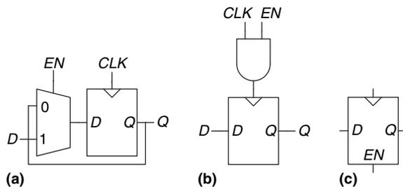
**Figure 3.10** Enabled flip-flop:
