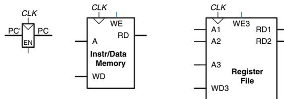
**Figure 7.16** State elements with unified instruction/data memory
