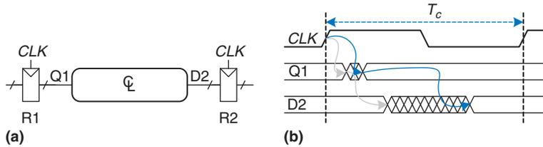
Figure 3.38 Path between registers and timing diagram
