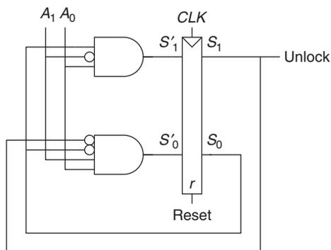
Figure 3.35 Circuit of found FSM for Example 3.9
