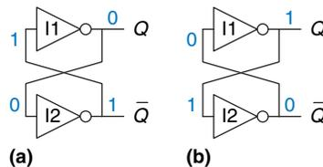
**Figure 3.2** Bistable operation of cross-coupled inverters
