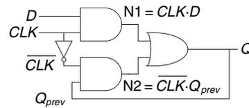
output,  $Q$ , given the two inputs,  $D$  and  $CLK$ , and the old state of the latch,  $Q_{prev}$ . Based on this truth table, he has derived Boolean equations. He obtains  $Q_{prev}$  by feeding back the output,  $Q$ . His design is shown in Figure 3.18. Does his latch work correctly, independent of the delays of each gate?
