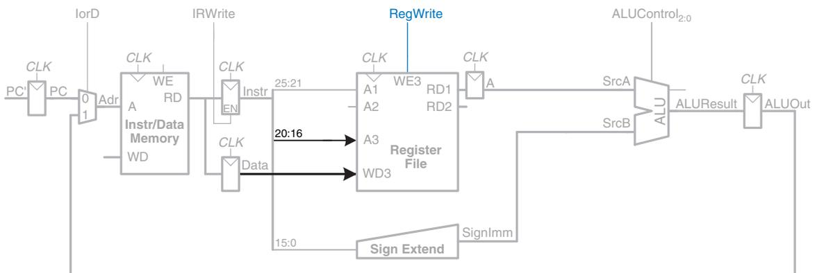
Figure 7.22 Write data back to register file
