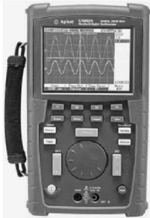
**Figure 16.16** Handheld digital storage oscilloscopes. Reproduced with permission of Fluke Corporation.
