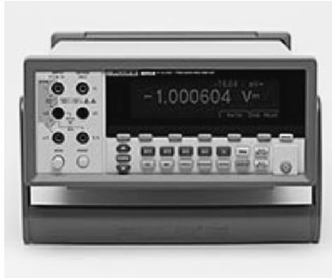
**Figure 16.10** Benchtop digital multimeter. Reproduced with permission of Fluke Corporation.
