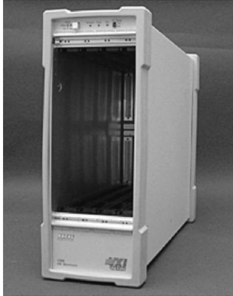
**Figure 16.42** VXI-bus instruments. Photo courtesy of National Instruments Corporation.
