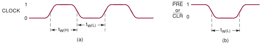
FIGURE 5-36 (a) Clock LOW and HIGH times; (b) asynchronous pulse width.
