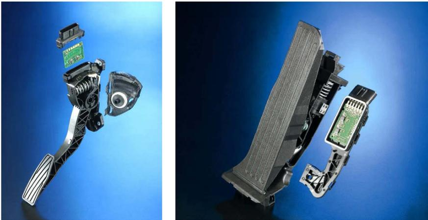
*Fig. 23 Acceleration Pedals with CIPOS-Sensors*
