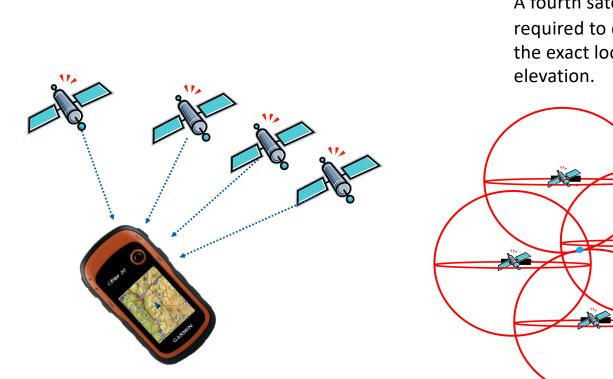
A fourth satellite is required to determine the exact location and
