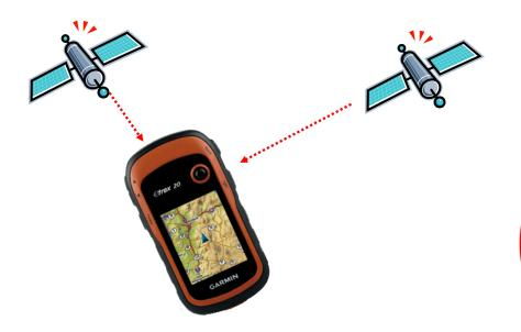
If the GPS receiver only obtains signals from 2 satellites, then it "knows" that it is located somewhere where these 2 spheres intersect
