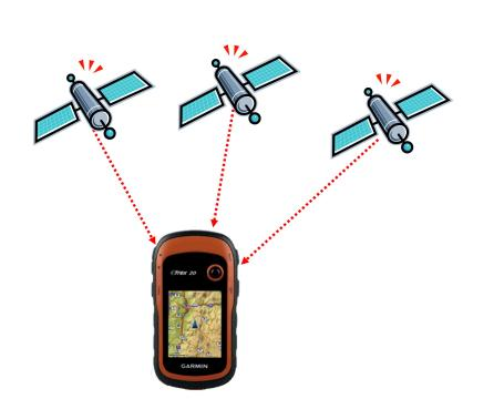
If the GPS receiver obtains signals from 3 satellites, then it "knows" that it is located somewhere where these 3 spheres intersect (2 points)
