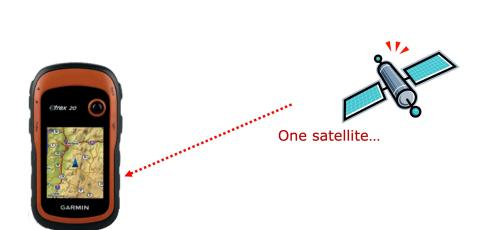
If the GPS receiver only obtains signals from 1 Satellite, then it "knows" that it is located somewhere on this sphere...
