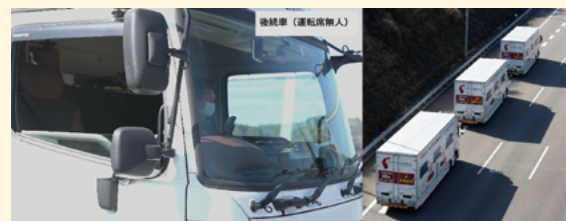
Unmanned rear vehicles in a convoy (Shin Tomei Expressway, February 22, 2021)
