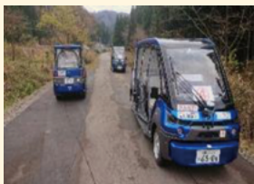
One remote driver operates three unmanned automated vehicles.
