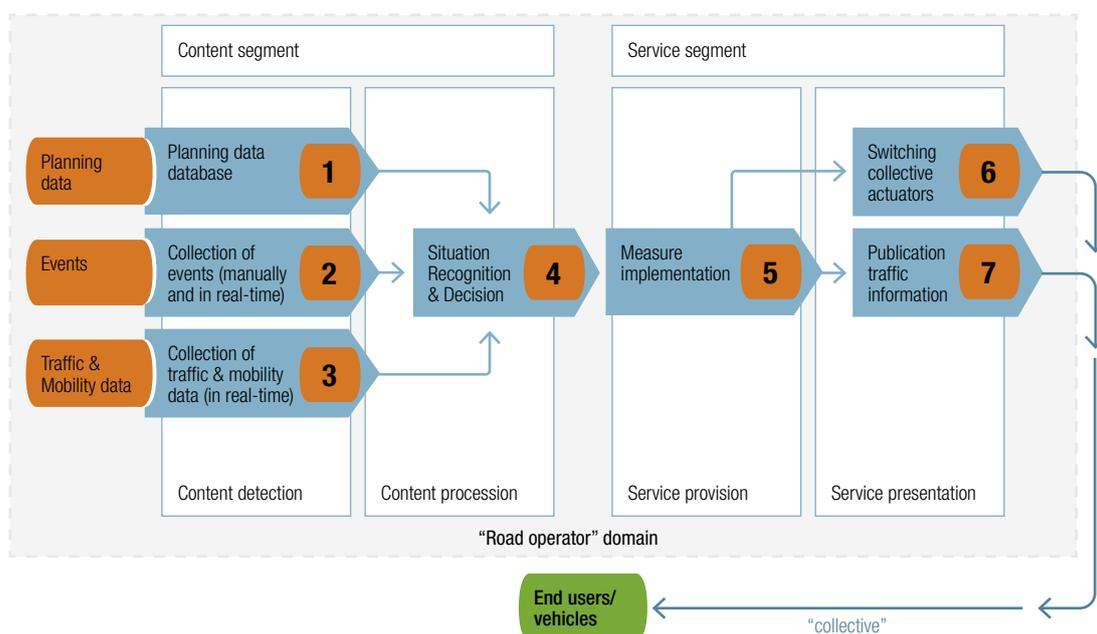
Figure 39 shows the approach of the basic value chain model for Traffic Management on the public road operator's side, based on the "TISA Value Chain Model". Traffic Management processes the gathered data and creates additional value of data using decision making mechanisms.
