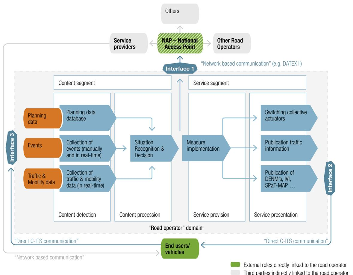
The centre of the diagram represents the road operator domain with the ITS service and its system boundary. The value chain overview - depicted in the background - is used as a symbol for the road operator processes. On the service boundary – depicted by a grey dotted line – we see three interfaces, which are served with two types of communication (network based communication, direct communication).
