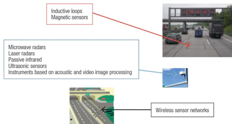
It is important to clarify that the technical equipment such as sensors, cameras, VMSs, etc., are used both for incident detection and warning as well as for the daily management of the network.
