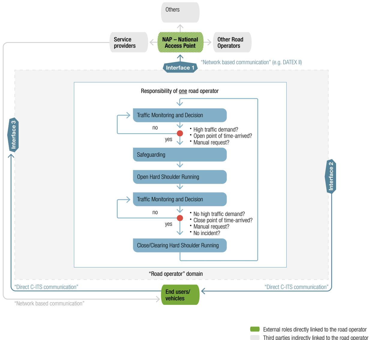
Hard Shoulder Running is carried out with a control algorithm or by using a manual request according to pre-determined traffic conditions such as high traffic demand.
