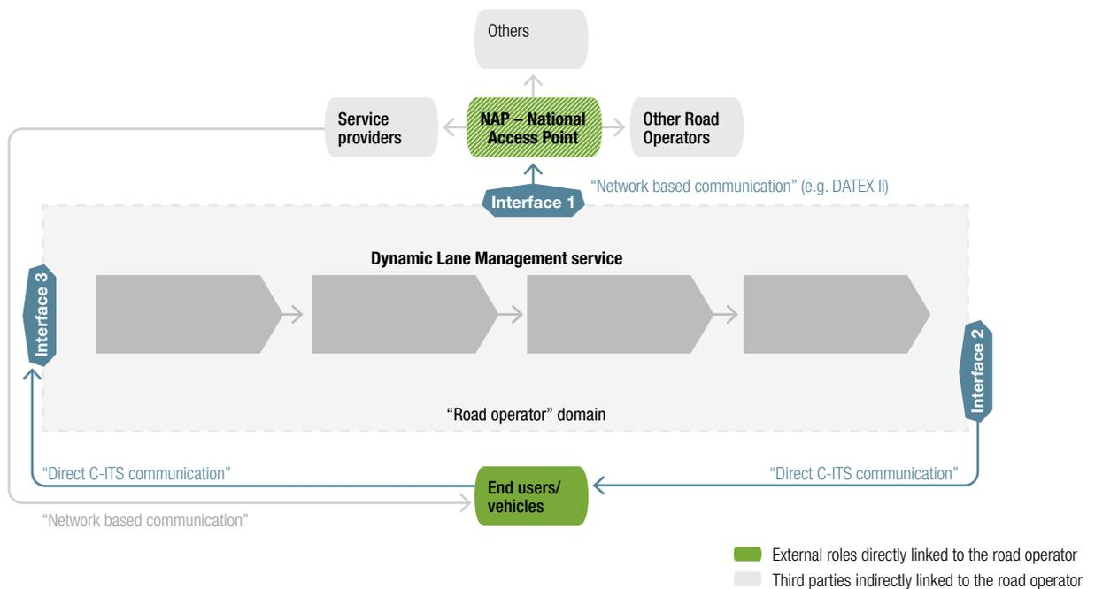
Figure 45 shows the typical functional and information architecture of the Dynamic Lane Management service.
