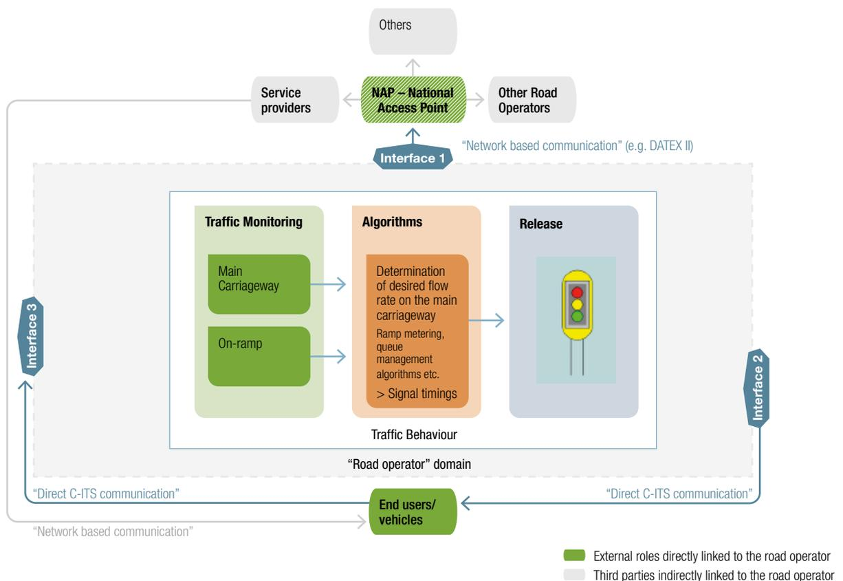
Cooperation with the adjacent network operators and their traffic control systems also need to be considered where appropriate. This can be achieved using a DATEX II reference profile.
