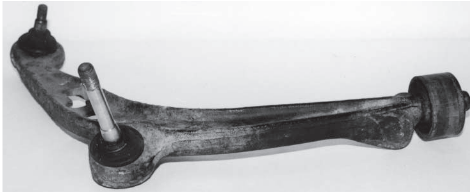
Figure 15.13 Lower wishbone from BMW Series 3 car
