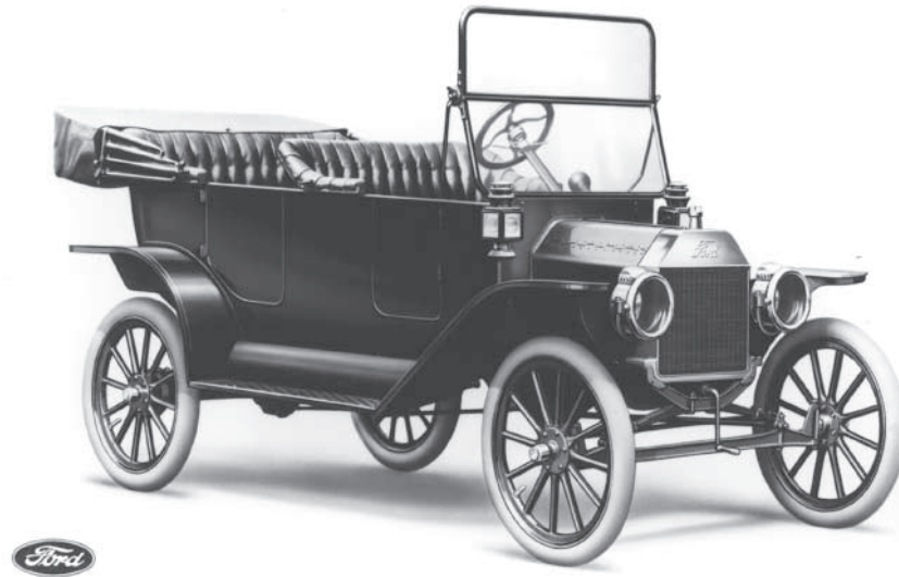
Figure 1.3 The Ford Model T. This example is from 1913. Note the single transverse front spring and the starting handle, which was the only means of starting. In addition to factory-built vehicles, independent coachbuilders used the Model T chassis as the basis for a wide range of bodywork styles, from trucks and charabanc buses to elegant coachbuilt family cars. The 2898cc petrol engine gave adequate power for use in quite large commercial vehicles. The spindly chassis was deceptively strong, being made of a vanadium steel alloy. (Photo courtesy of Ford Motor Company Ltd.)
