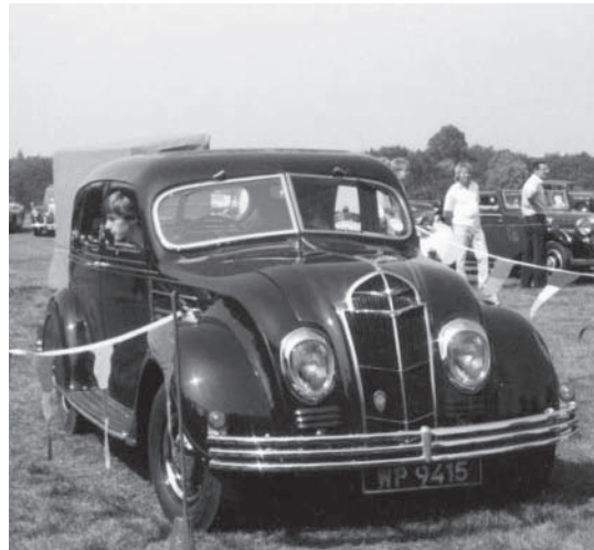
Figure 1.10 The Chrysler Airflow incorporated a number of advanced features for the 1930s, including aerodynamic styling and semi-unitary construction. Though popular now at shows because of its rarity, it was a commercial failure in its time. Note the split windscreen and almost blended headlamps.
