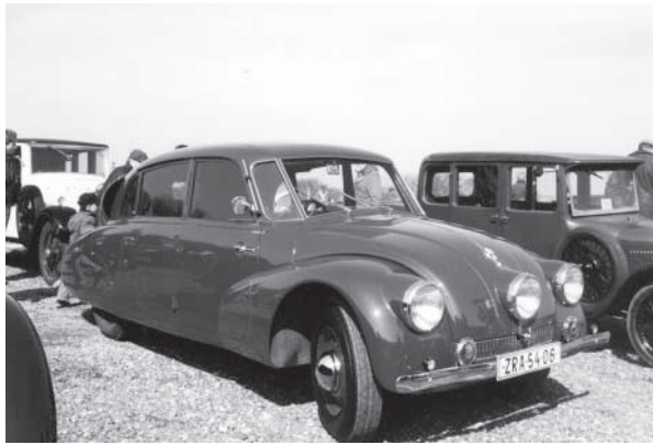
Figure 1.9 True aerodynamic design. The Czech Tatra of 1937 with air-cooled rear-engined V-8 was a very advanced vehicle for its time.
