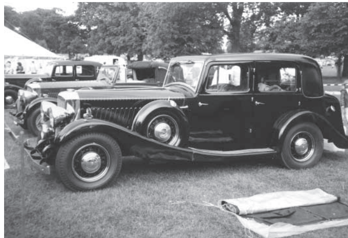
Figure 1.5 This 1935 Railton Carbodies saloon combines classic features of both American and British design. The engine is a Hudson unit with a three-speed crash gearbox. Sixteen-inch American size wheels are used, but the hand-built coachwork with ash frame, aluminium panelling and steel wings is typically British. The long bonnet is actually justified in this case, because of the straight-eight 4.2 litre engine. Note the small boot, which had only recently evolved from a separate trunk. Windscreen wipers had been standard for several years, but the flat front screen could still be hinged open.
