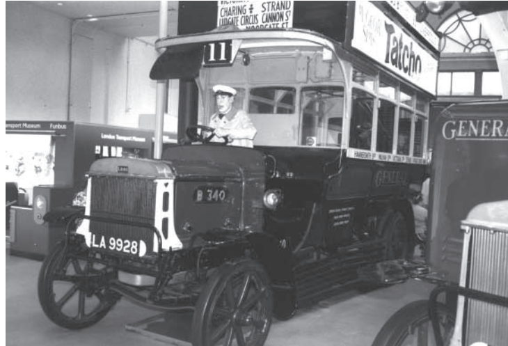
Figure 1.12 A 1911 London B-type bus. Petrol-engined buses soon displaced the earlier horsedrawn vehicles. Note how the driver and upper deck passengers are totally exposed to the weather. The tyres are solid rubber. (From the collection of the London Transport Museum.)
