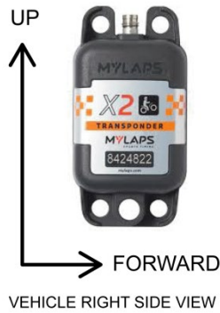
Figure B-67: Transponder Orientation
