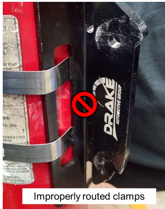
Figure B-52: Incorrect routing of hose clamps.
