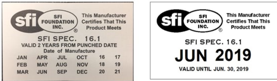
Figure B-30: Driver Harness, SFI Tag, Old Style (Left), New Style (Right)
