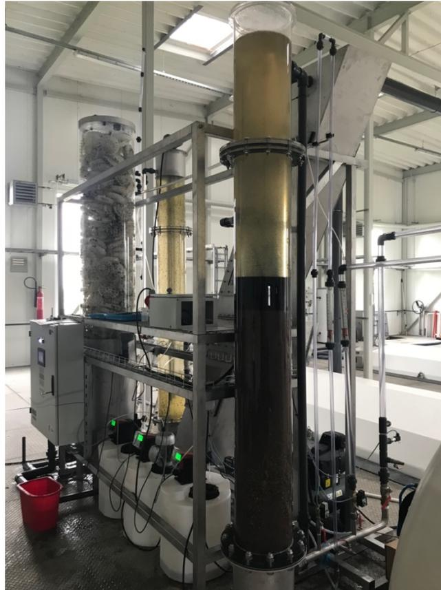
*Figure 12. Test device set up as part of the BEST (Better Efficiency for Industrial Sewage Treatment) project funded under INTERREG Baltic Sea Region Programme. The configuration in the picture consists of the sand filter combined with GAC.*
