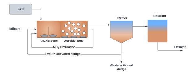
Figure 8. Dosing of PAC directly into the existing activated sludge process. Final filters remove the residues of TSS, which contain also small concentrations of PAC that has adsorbed the micropollutants.
