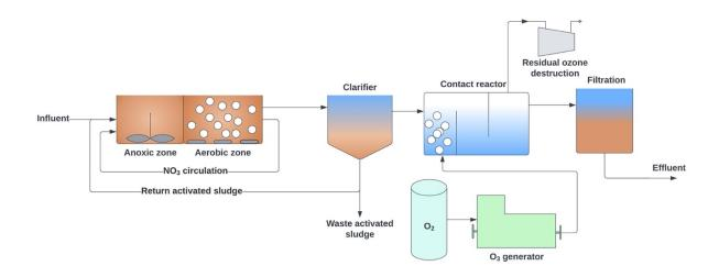
*Figure 14. Removal of micropollutants at the WWTP by applying ozonation.*
