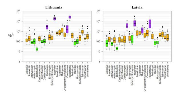
Figure 3. API concentrations measured in the influent of the WWTPs in Lithuania (left) and in Latvia (right). 2 samplings per WWTP at 8 WWTPs per country (n = 16 per country; C < LOQ = LOQ2). Colours highlight different concentration levels with respect to the median concentrations > 1000 ng/l (purple), 100-1000 ng/l (amber), and < 100 ng/l (green).
