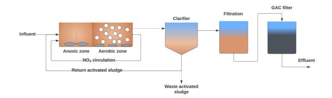
Figure 11. Using the GAC filter to remove micropollutants. The filter before GAC is optional and depends on the local circumstances (e.g., how much of TSS is carried out from the final clarifiers).
