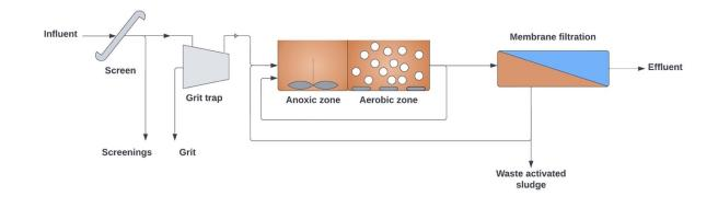
Figure 16. Membrane bioreactor. Activated sludge is separated from wastewater by membrane filtration, not by settling. This process also separates most of the hazardous compounds.
