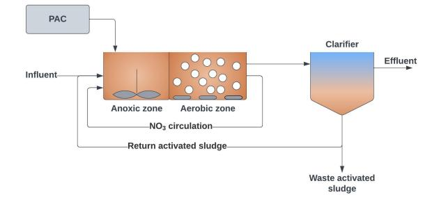
Figure 7. Dosing of PAC directly into the existing activated sludge process. Micropollutants are removed with waste activated sludge.
