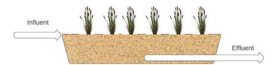
Figure 17. Simplified buried filter. Wastewater from biological treatment is discharged into the buried filter for post-treatment.
