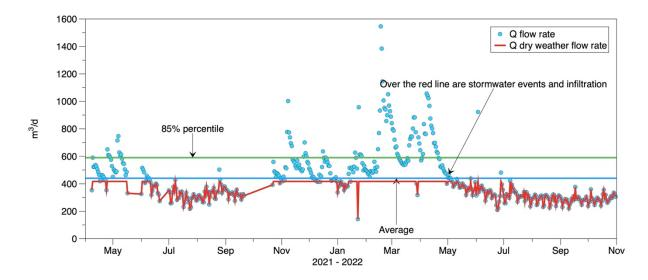
*Figure 5. A WWTP flow rate analysis prepared to calculate the hydraulic load underlying the sizing of the post-treatment.*
