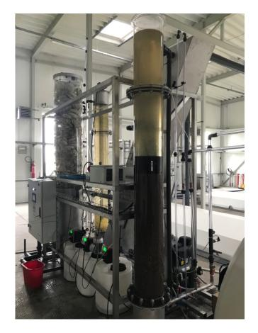
Figure 12. Test device set up as part of the BEST (Better Efficiency for Industrial Sewage Treatment) project funded under INTERREG Baltic Sea Region Programme. The configuration in the picture consists of the sand filter combined with GAC.
