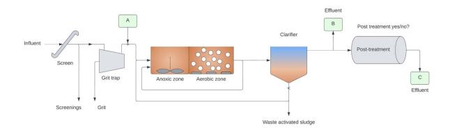
*Figure 2. Micro-pollutant sampling points: A - influent, B - effluent and, where post-treatment is available, an additional sample is taken from point C.*
