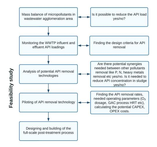
Figure 6. The process of selecting post-treatment technology with emphasis on API removal, while analysing also potential synergies with the treatment of any other pollutants using the same or combined types of solutions.
