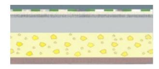
new surface overlay > 50mm BITUTEX® - Composite compensation layer
