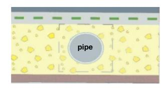
Repair above supply trenches BITUTEX® - Composite
