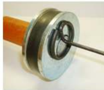
The flat surface of the fasteners sits flush on the magnetic head of the Pin Pounder.
