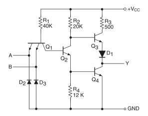
Figure 5.17 NAND gate in the low-power TTL.
