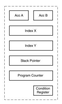
Figure 14.12 Accumulator-based processor architecture.
