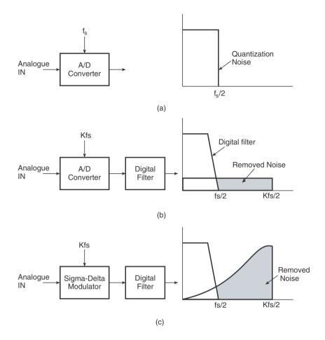
**Figure 12.38** (a) Quantization noise spectrum with sampling at the Nyquist rate, (b) the quantization noise spectrum with oversampling and (c) the quantization noise spectrum with oversampling in a sigma-delta converter.
