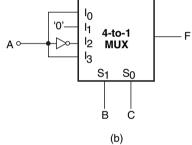
Figure 8.8 Hardware implementation of the Boolean function given by equation (8.3).
