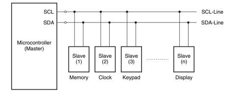
Figure 14.7 Master–slave configuration – one I<sup>2</sup>C master and multiple slaves.
