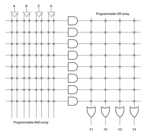
Figure 9.11 Internal architecture of a PLA device.
