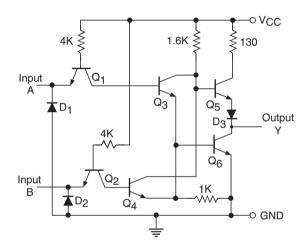
Figure 5.9 NOR gate in the standard TTL.
