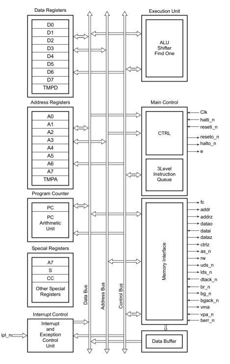
Figure 13.16 Block diagram of the 68000 microprocessor.
