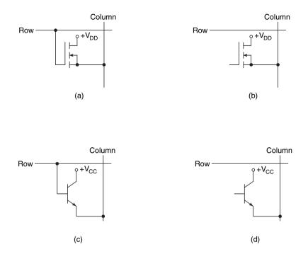
Figure 15.16 Basic cell connection of a mask-programmed ROM.
