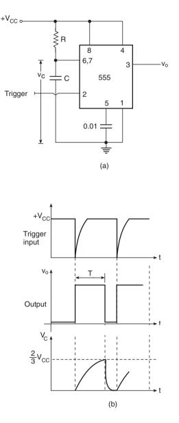
Figure 10.11 (a) Monostable multivibrator using timer 555 and (b) monostable multivibrator relevant waveforms.
