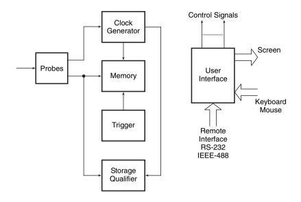
Figure 16.35 Logic analyser architecture.
