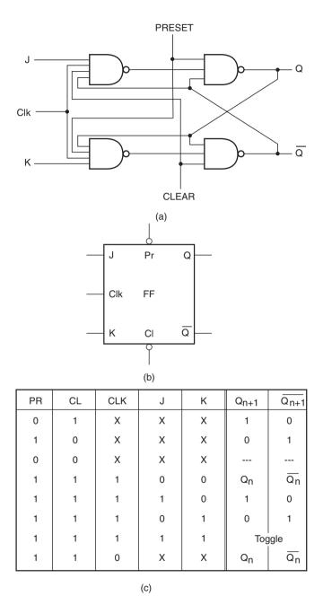
Figure 10.29 *J-K* flip-flop with PRESET and CLEAR inputs.
