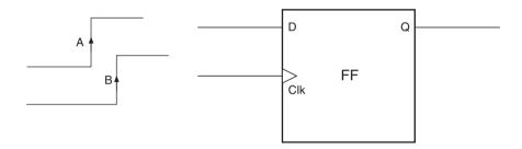
Figure 10.51 Detection of the sequence of edges.
