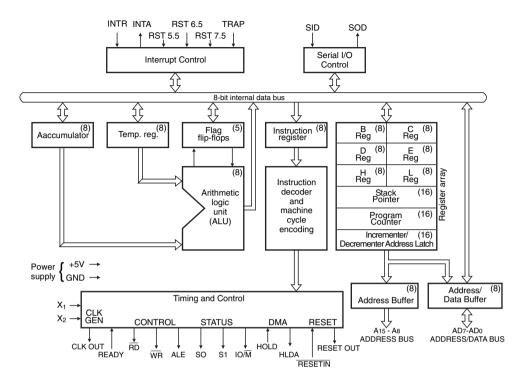
Figure 13.12 Block diagram of 8085.
