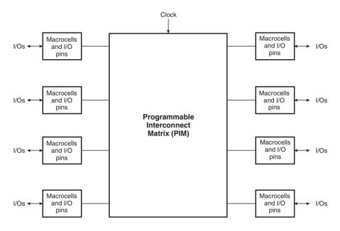
Figure 9.40 FLASH-370 CPLD architecture.
