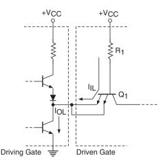
Figure 5.27 Input loading in the case of LOW tied inputs of NAND and AND gates.
