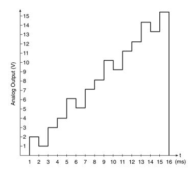
Figure 12.13 Staircase waveform (example 12.4).
