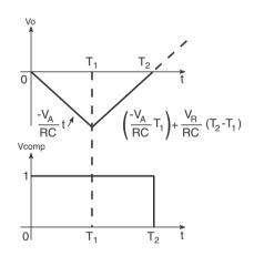
Figure 12.37 Relevant waveforms in a dual-slope A/D converter.
