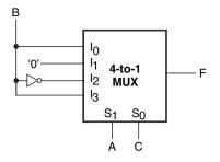
Figure 8.10 Hardware implementation using a 4-to-1 multiplexer.
