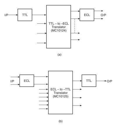
Figure 5.64 TTL-to-ECL and ECL-to-TTL interfaces.
