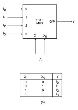
Figure 8.1 (a) 4-to-1 multiplexer circuit representation and (b) 4-to-1 multiplexer truth table.
