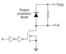
Figure 5.47 CMOS inverter with an open drain output.
