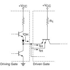
Figure 5.26 Input loading in the case of HIGH tied inputs of NAND and AND gates.
