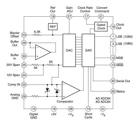
Figure 12.45 Internal architecture/pin connection diagram of AD ADC-84/ADC-85/AD-5240.
