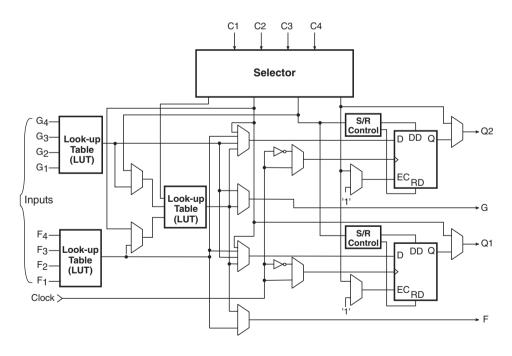
Figure 9.28 Logic block architecture of the XC4000 FPGA from Xilinx.
