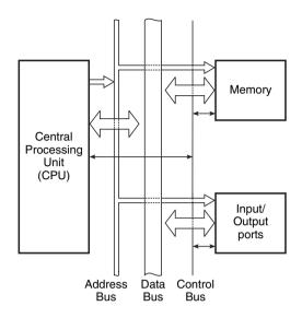
Figure 15.1 Block schematic of a typical computer.
