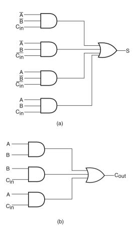
Figure 7.9 Logic circuit diagram of a full adder.
