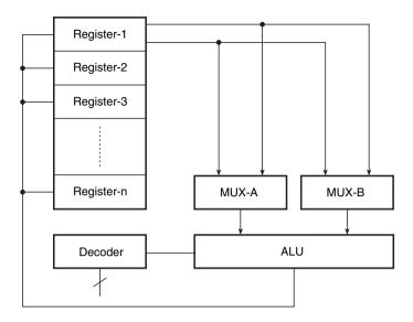
Figure 14.13 Register-based processor architecture.
