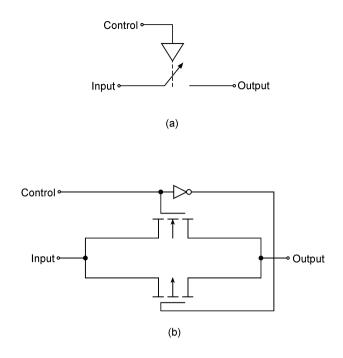
Figure 5.45 Transmission gate.
