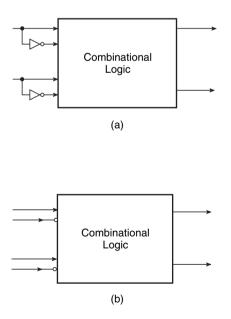
Figure 7.2 Combinational circuit with normal and complemented inputs.
