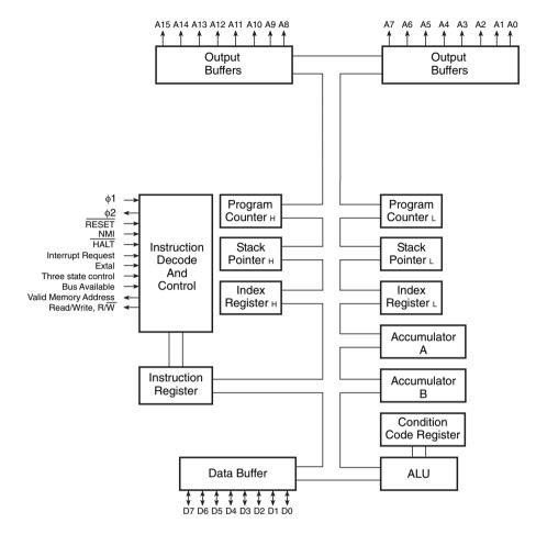
Figure 13.13 Block diagram of 6800.
