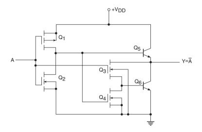
Figure 5.55 BiCMOS inverter.
