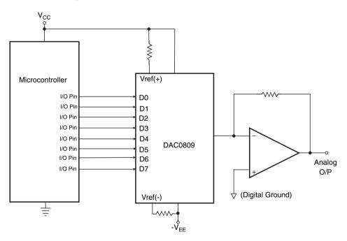
Figure 14.36 Interface of a D/A with a microcontroller.
