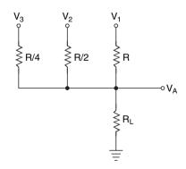
Figure 12.1 Simple resistive network for D/A conversion.
