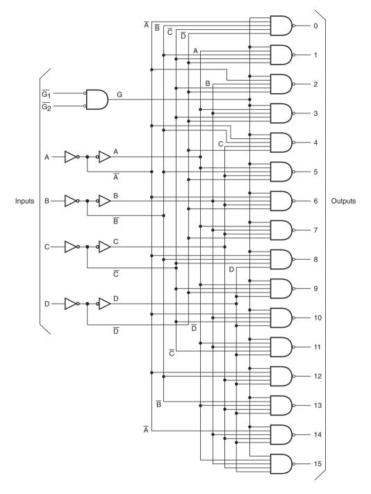
Figure 11.19 Logic diagram of IC 74154.
