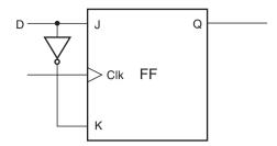
Figure 10.40 *J-K* flip-flop as a *D* flip-flop.
