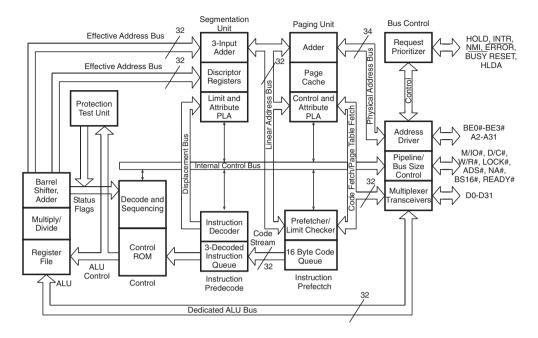
Figure 13.17 Block diagram of the 80386 microprocessor.
