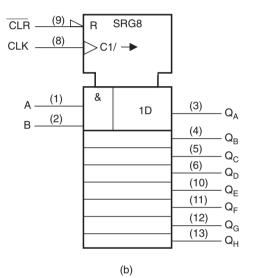
Figure 11.53 IEEE/ANSI notation for (a) IC 7491 and (b) IC 74164.
