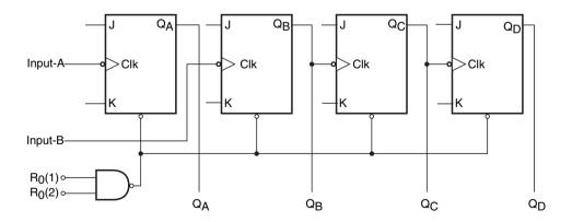
Figure 11.4 Logic diagram of IC 74293.
