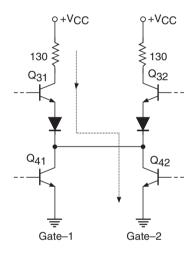
Figure 5.15 Totem-pole output gates tied at the output.
