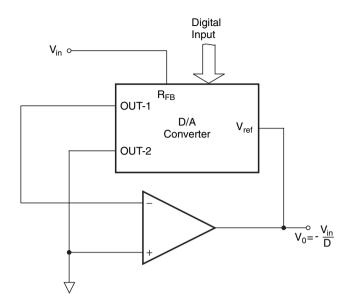
Figure 12.20 Digitally controlled divider.
