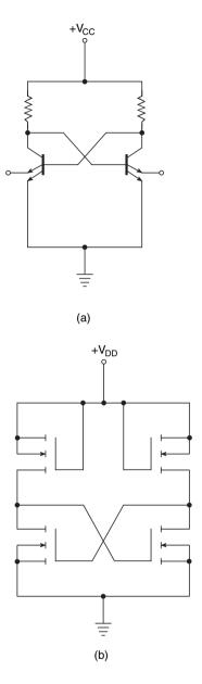
Figure 15.5 (a) Basic bipolar memory cell and (b) a basic MOS memory cell.
