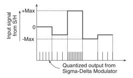
Figure 12.40 Generation of a one-bit data stream.
