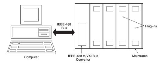
Figure 16.43 VXI instrument-PC interface using IEEE-488.
