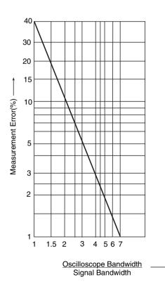
Figure 16.17 Measurement error as a function of oscilloscope bandwidth.
