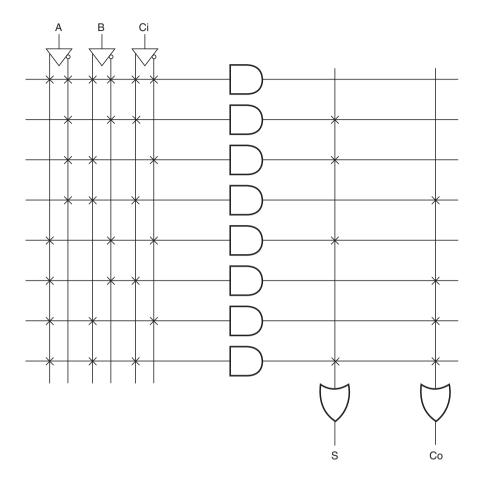
Figure 9.15 Solution to problem 9.2 using a PLA.
