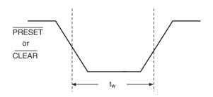
Figure 10.46 Asynchronous input active pulse width.
