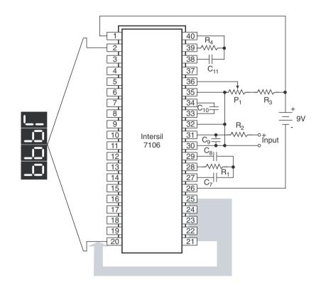
Figure 12.48 Application circuit using ICL 7106.
