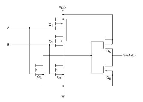
Figure 5.40 Two-input OR in CMOS.
