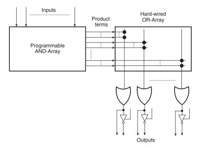
Figure 9.18 Generalized PAL device.
