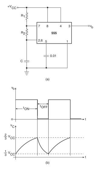
**Figure 10.10** (a) Astable multivibrator using timer IC 555, (b) astable multivibrator relevant waveforms and (c, d) modified versions of the astable multivibrator using timer IC 555.
