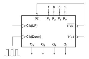
Figure 11.13 Presettable four-bit counter.
