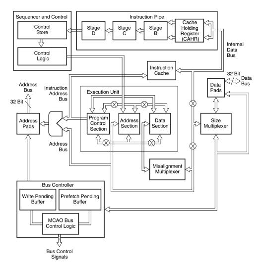
Figure 13.18 Block diagram of 68020.
