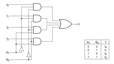
Figure 8.5 Logic diagram of a 4-to-1 multiplexer.
