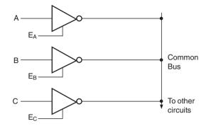
Figure 4.28 Paralleling of tristate inverters.
