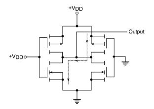
Figure 5.46 CMOS inverters with shorted outputs.
