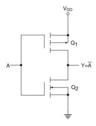
Figure 5.34 CMOS inverter.
