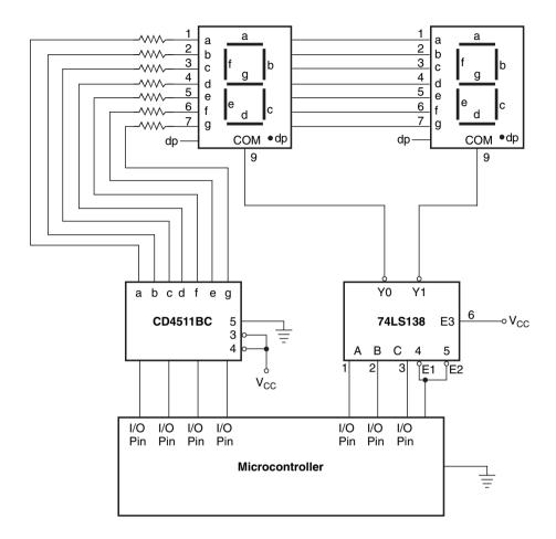
Figure 14.32 Multiplexed circuit for two CC displays.
