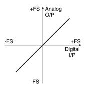
Figure 12.7 Bipolar-output D/A converter transfer characteristics.
