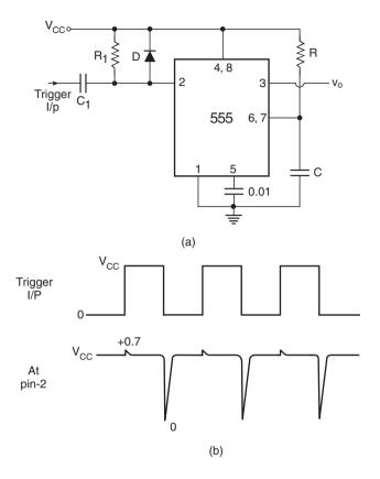
Figure 10.12 555 monoshot triggering on trailing edges.
