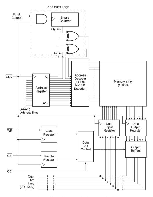
Figure 15.9 Architecture of a 16K ×8 synchronous SRAM.
