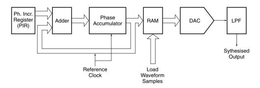
Figure 16.32 Arbitrary waveform generator architecture.
