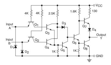
Figure 5.11 OR gate in the standard TTL.
