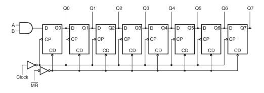
Figure 11.38 Logic diagram of IC 74164.
