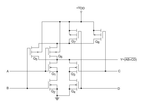
Figure 5.43 Two-wide, two-input AND-OR-INVERT gate in CMOS.
