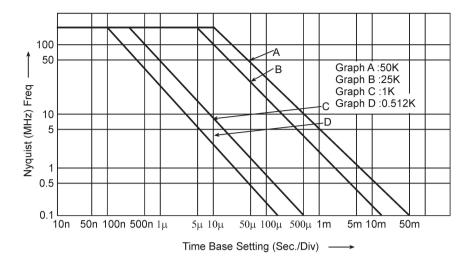
Figure 16.18 Effective sampling rate – time-base setting graph.
