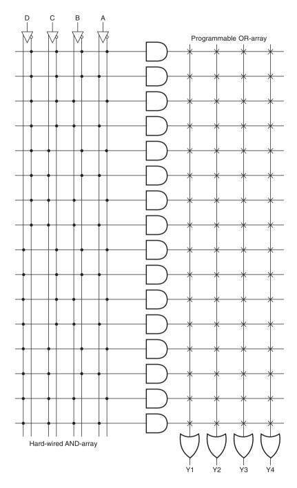
Figure 9.3 Internal architecture of a PROM.
