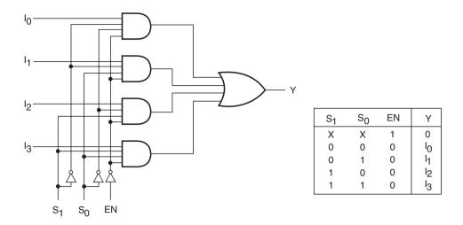
Figure 8.7 4-to-1 multiplexer with an ENABLE input.
