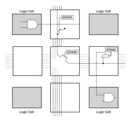
Figure 9.32 SRAM-controlled interconnect.
