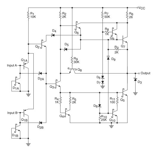
Figure 5.22 NAND gate in the AS-TTL.
