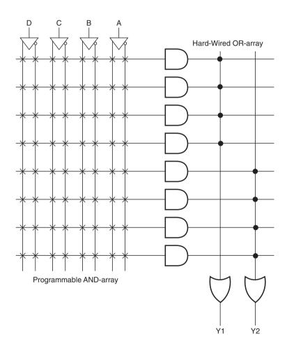
Figure 9.5 Internal architecture of a PAL device.
