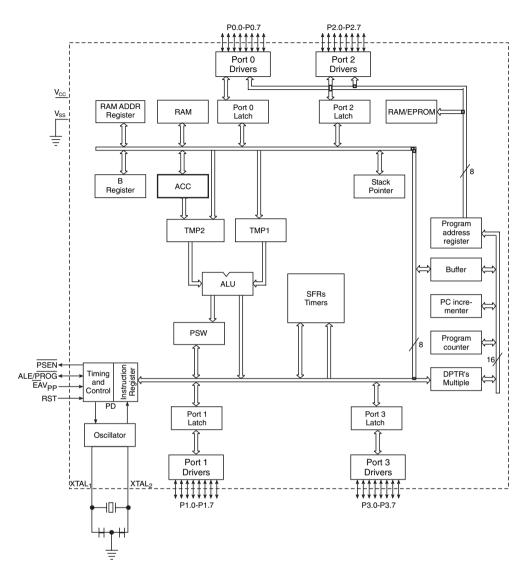
Figure 14.16 Architecture of the 80C51 microcontroller family.
