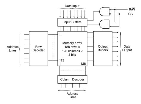
Figure 15.7 Typical architecture of a 16K×8 asynchronous SRAM.
