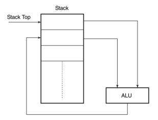
Figure 14.14 Stack-based processor architecture.
