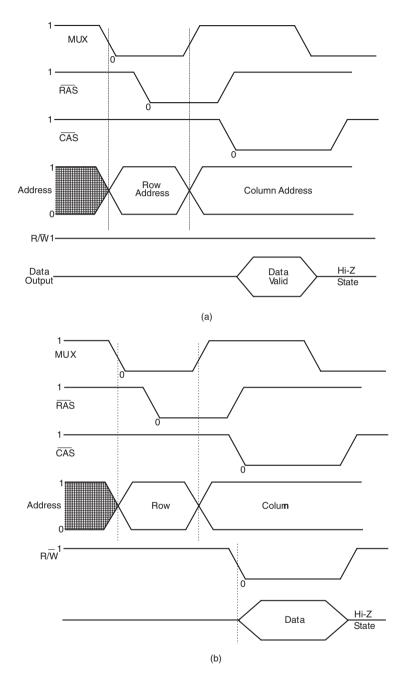
Figure 15.12 (a) Timing diagrams for a READ operation and (b) timing diagrams for a WRITE operation.
