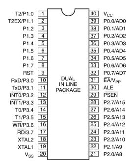
Figure 14.17 PIN connection diagram in the 40-pin DIP package.
