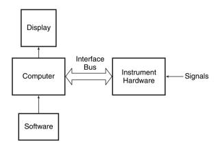
Figure 16.40 Components of a virtual instrument.
