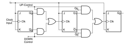
Figure 11.10 Four-bit UP/DOWN counter.
