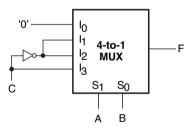
Figure 8.9 Hardware implementation using a 4-to-1 multiplexer.
