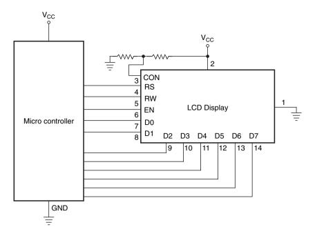
Figure 14.34 LCD display interface with a microcontroller.
