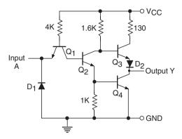
Figure 5.8 Inverter in the standard TTL.
