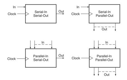
Figure 11.34 Circuit representation of shift registers.
