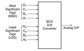
Figure 12.10 BCD-input D/A converter.
