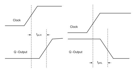
Figure 10.44 Propagation delay.
