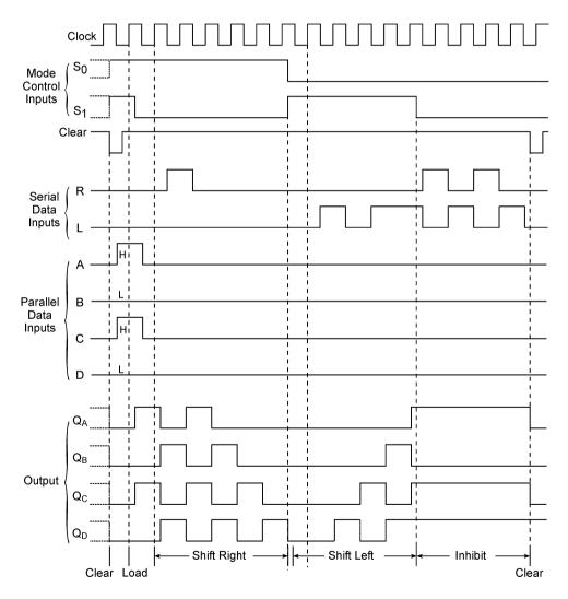
Figure 11.44 Timing waveforms of IC 74194.
