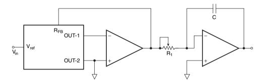
Figure 12.22 Non-inverting programmable integrator.
