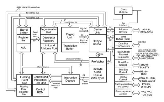
Figure 13.19 Internal architecture of 80486DX.
