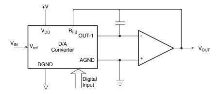
Figure 12.19 Digitally controlled audio signal attenuator.
