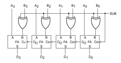
Figure 7.19 Four-bit adder-subtractor.
