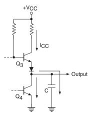
Figure 5.29 Current transients and power supply decoupling.
