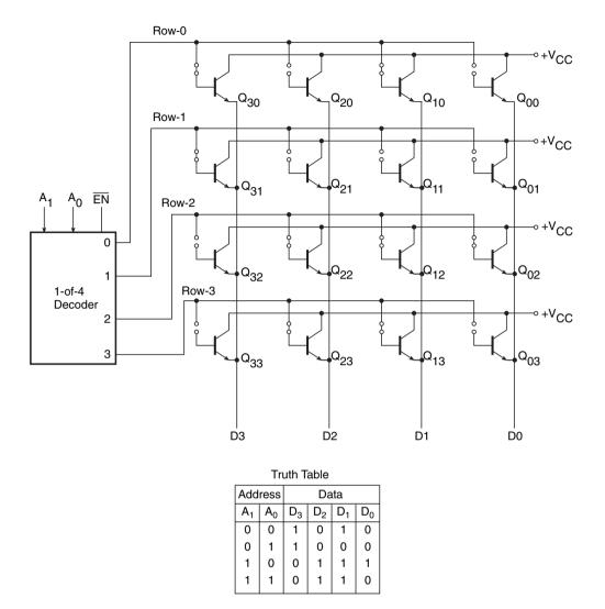
Figure 15.17 Internal structure of a  $4 \times 4$  bipolar mask-programmed ROM.
