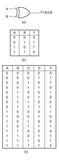
**Figure 4.12** (a) Circuit symbol of a two-input EXCLUSIVE-OR gate, (b) the truth table of a two-input EXCLUSIVE-OR gate and (c) the truth table of a four-input EXCLUSIVE-OR gate
