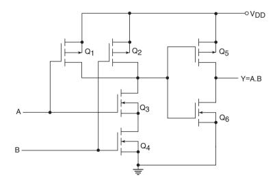
Figure 5.39 Two-input AND in CMOS.
