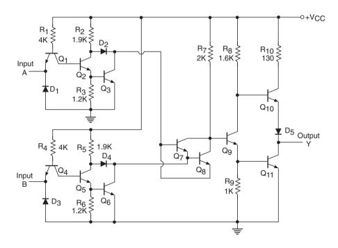
Figure 5.12 EX-OR gate in the standard TTL.
