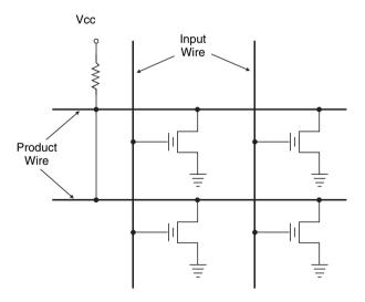
Figure 9.30 Floating-gate transistor interconnect.
