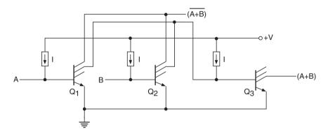
Figure 5.60 Wired logic in  $I^2L$ .
