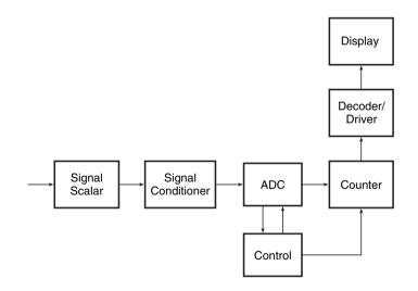
Figure 16.8 Block schematic of a digital meter.
