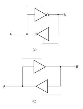
Figure 4.41 (a) Inverting transceivers and (b) noninverting transceivers.
