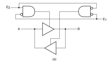
Figure 4.42 Tristate noninverting transceiver.
