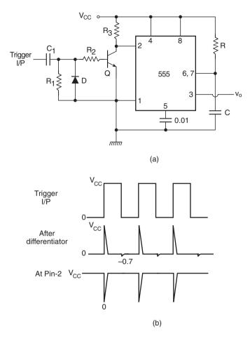
Figure 10.13 555 monoshot triggering on leading edges.
