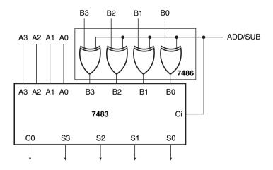
Figure 16.7 Adder–subtractor circuit (example 16.5).
