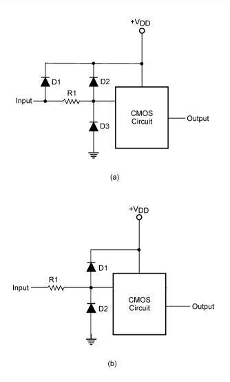
Figure 5.49 (a) Input protection circuit-metal-gate devices and (b) input protection circuit-silicon-gate devices.
