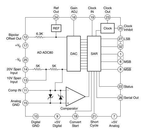
Figure 12.44 Internal architecture/pin connection diagram of AD ADC 80.
