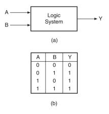
Figure 4.1 Two-input logic system.
