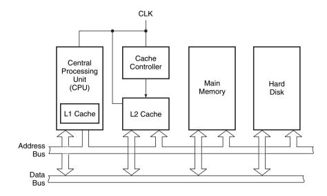
Figure 15.13 Cache memory in a computer system.
