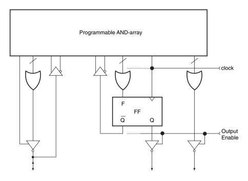
Figure 9.20 Output logic arrangements in a PAL device.
