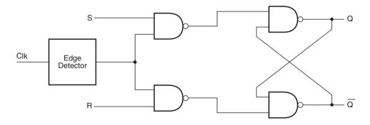
Figure 10.23 Edge-triggered R-S flip-flop.
