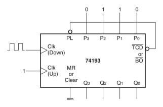
Figure 11.23 Presettable counter (example 11.7).
