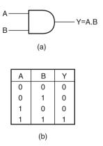
Figure 4.7 Two-input AND gate.
