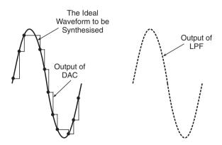
Figure 16.30 Direct digital synthesis – relevant waveforms.
