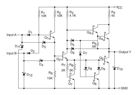
Figure 5.23 NAND gate in the FAST TTL.
