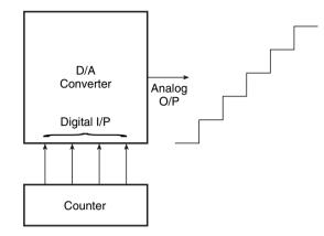
Figure 12.5 Monotonocity in a D/A converter.
