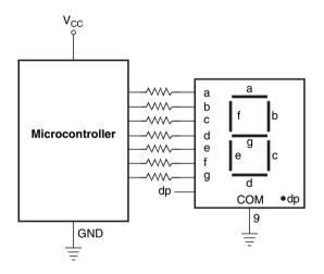
Figure 14.31 Direct circuit connection for CA display.
