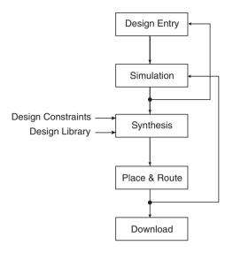
Figure 9.34 Programmable logic design and development process.
