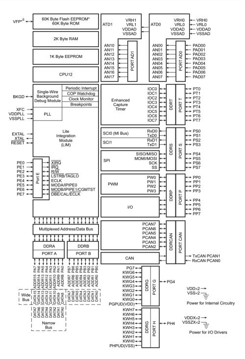
Figure 14.23 Architecture of the 68HC12 family of microcontrollers.
