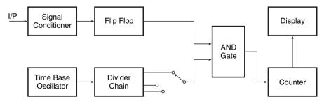
**Figure 16.22** Time period measurement using a frequency counter.
