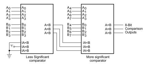
Figure 7.37 Cascading of individual magnitude comparators.
