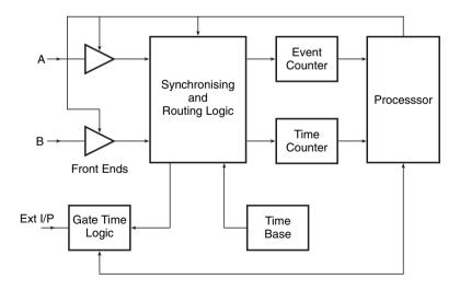
Figure 16.23 Reciprocal counter architecture.
