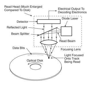
Figure 15.35 Use of a laser beam for CD READ operation.
