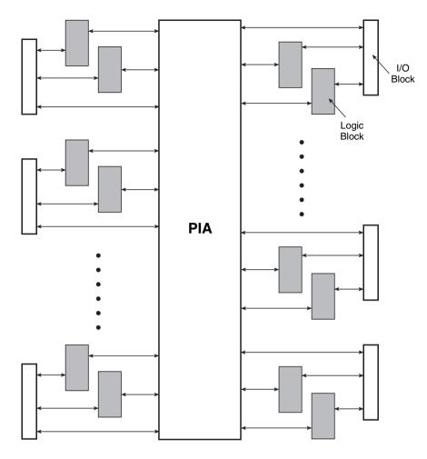
Figure 9.38 MAX-7000 series CPLD architecture.
