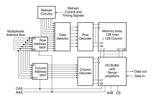
Figure 15.11 Architecture of a  $16K \times 1$  DRAM.
