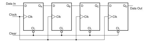
Figure 11.35 Serial-in, serial-out shift register.
