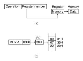
Figure 13.8 Register indirect addressing mode.
