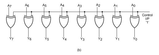
Figure 7.18 (a) One-bit controlled inverter and (b) eight-bit controlled inverter.
