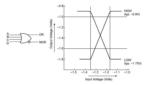
Figure 5.33 ECL input/output characteristics.
