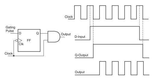
Figure 10.50 Flip-flop synchronization.
