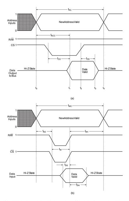
Figure 15.8 (a) Timing diagram during a READ operation and (b) the timing diagram during a WRITE operation.
