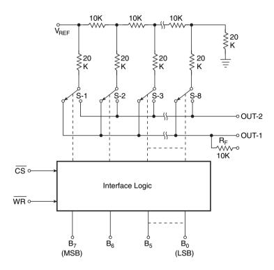
Figure 12.18 Functional diagram of AD 7524.
