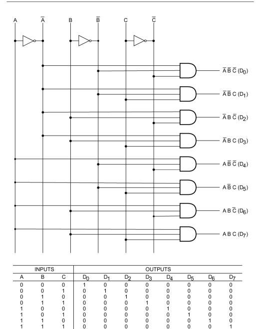
Figure 8.20 Logic diagram of a 3-to-8 line decoder.
