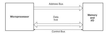
Figure 13.1 Microprocessor-based system.
