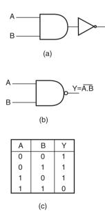
**Figure 4.15** (a) Two-input NAND implementation using an AND gate and a NOT circuit, (b) the circuit symbol of a two-input NAND gate and (c) the truth table of a two-input NAND gate.
