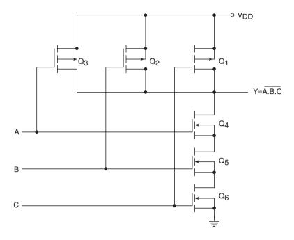
Figure 5.36 Three-input NAND in CMOS.
