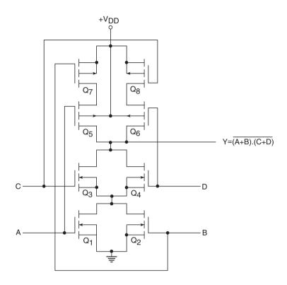
Figure 5.44 Two-wide, two-input OR-AND-INVERT gate.
