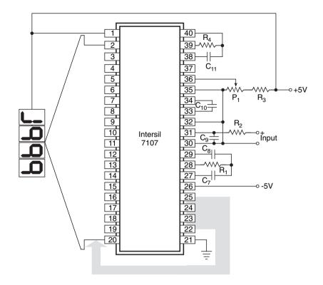
Figure 12.49 Application circuit using ICL 7107.
