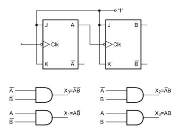
Figure 11.17 MOD-4 counter with decoding gates.
