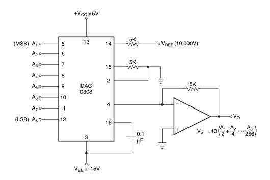
Figure 12.15 DAC-0808 wired as a voltage-output D/A converter.
