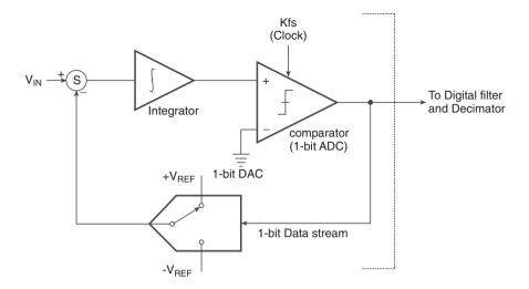
Figure 12.39 Block schematic representation of a delta modulator.
