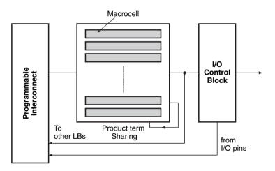
Figure 9.25 Logic block structure.
