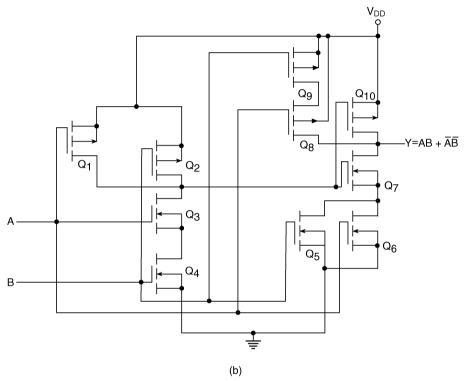
Figure 5.42 Two-input EX-NOR in CMOS.
