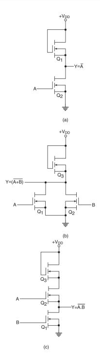
Figure 5.58 (a) NMOS logic circuit inverter, (b) NMOS logic two-input NOR and (c) NMOS logic two-input NAND.
