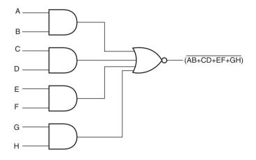
Figure 4.31 Four-wide, two-input AND-OR-INVERT gate.
