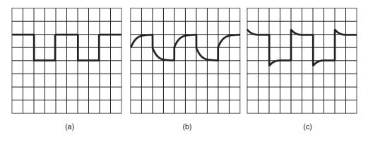
Figure 16.20 Probe compensation.
