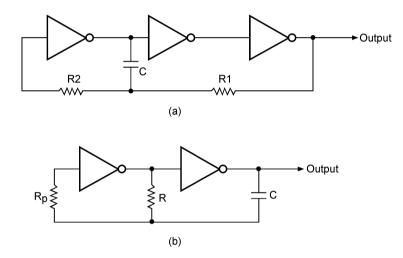
Figure 4.53 Square-wave oscillator with external components.
