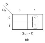
Figure 10.39 D flip-flop.
