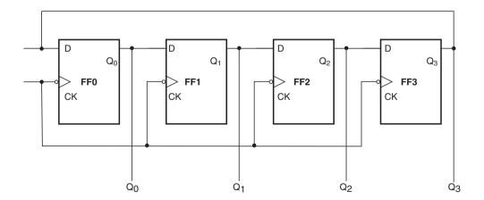
Figure 11.45 Four-bit ring counter.
