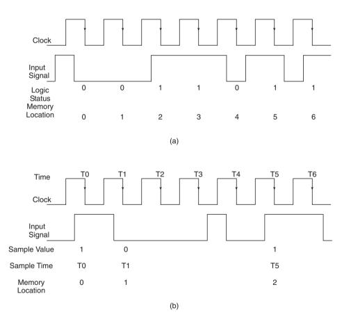
Figure 16.36 Logic analyser - relevant waveforms.
