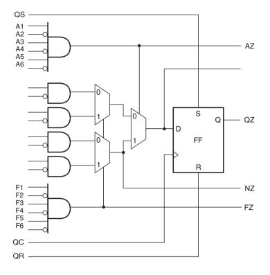
Figure 9.42 Quicklogic FPGA logic block.
