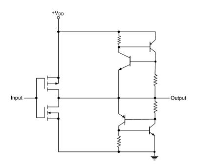
Figure 5.50 CMOS inverter with parasitic elements.
