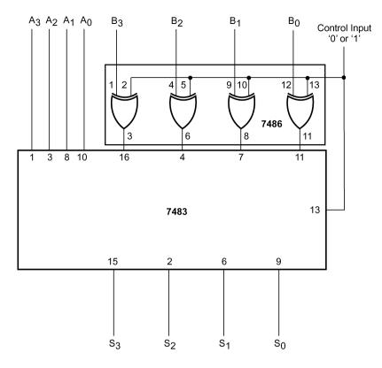
Figure 7.20 Four-bit adder-subtractor.
