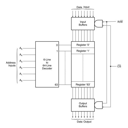
Figure 15.6 Typical architecture of a 64×8 asynchronous SRAM.
