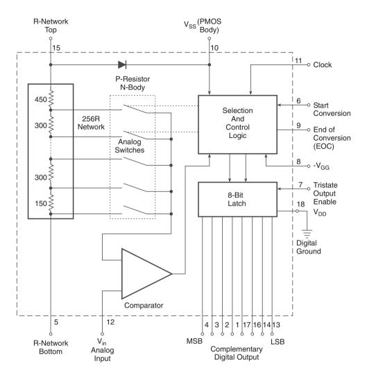
Figure 12.41 Internal architecture of AD 0800.
