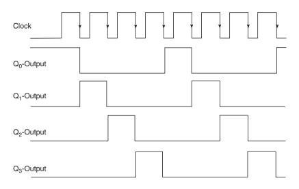
Figure 11.46 Timing waveforms of the four-bit ring counter.
