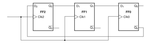
Figure 16.5 Three-bit shift counter (example 16.4).
