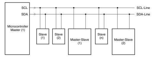
Figure 14.8 Master-slave configuration - multiple-master support arrangement.
