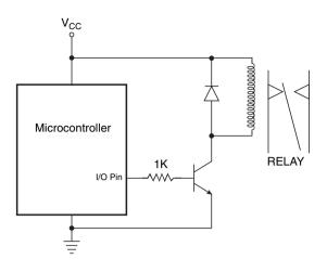
Figure 14.26 Interfacing an electromechanical relay to a microcontroller.
