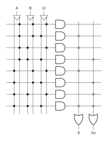
Figure 9.14 Solution to problem 9.2 using a PROM.
