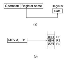
Figure 13.7 Register direct addressing mode.
