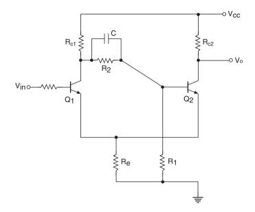
Figure 10.2 Schmitt trigger circuit.
