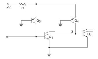
**Figure 5.59** Integrated injection logic (I<sup>2</sup>L).
