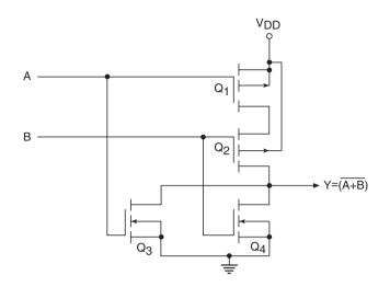
Figure 5.37 Two-input NOR in CMOS.
