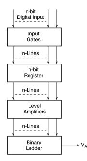
Figure 12.3 Block schematic representation of a D/A converter.
