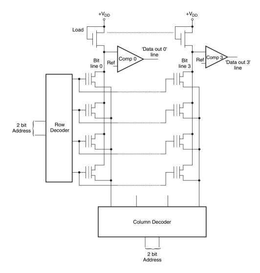
Figure 15.20 Basic array of  $4 \times 4$  flash memory.
