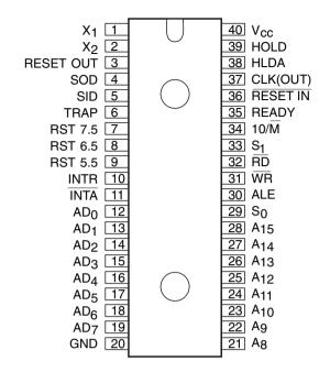
Figure 13.11 Pin-out configuration of 8085.
