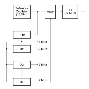
Figure 16.25 Frequency synthesizer architecture – direct frequency synthesis.
