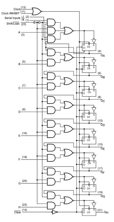
Figure 11.42 Logic diagram of IC 74199.
