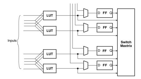
Figure 9.29 Logic block architecture of an AT&T FPGA.
