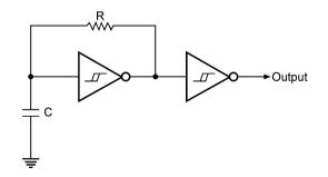
Figure 4.54 Schmitt inverter based oscillator.
