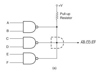
Figure 4.26 WIRE-AND connection with open collector/drain devices.
