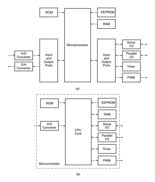
Figure 14.1 Microprocessor versus microcontroller: (a) microprocessor configuration; (b) microcontroller configuration.
