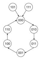
Figure 11.25 State transition diagram.
