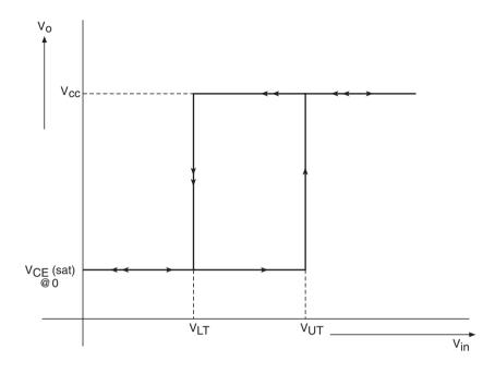
Figure 10.3 Transfer characteristics of a Schmitt trigger.
