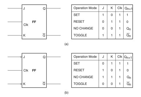
Figure 10.26 (a) J-K flip-flop active HIGH inputs and (b) J-K flip-flop active LOW inputs.
