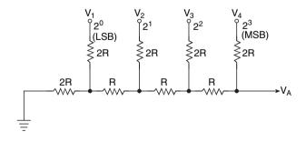
Figure 12.2 Binary ladder network for D/A conversion.
