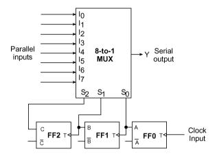
Figure 8.11 Multiplexer for parallel-to-serial conversion.
