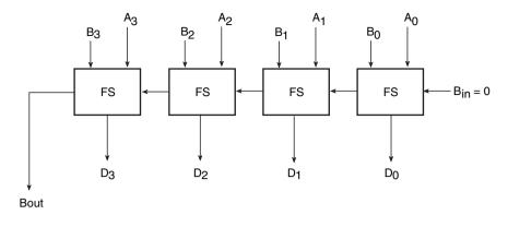
Figure 7.17 Four-bit subtractor.
