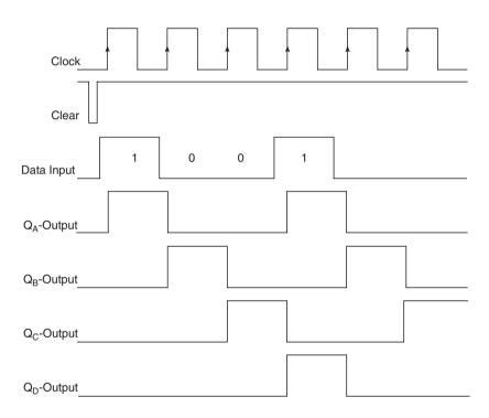
Figure 11.36 Timing waveforms for the shift register of Fig. 11.35.
