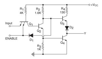
Figure 5.16 Tristate inverter in the TTL.
