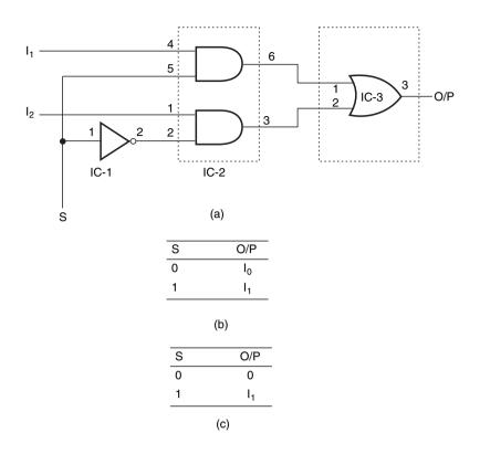
Figure 16.2 Combinational circuit (example 16.2).
