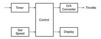
Figure 14.2 Microcontroller-based car cruise control.
