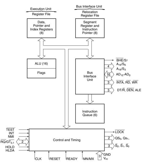
Figure 13.15 Block diagram of 8086.
