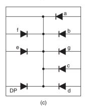
Figure 2.1 Seven-segment displays.
