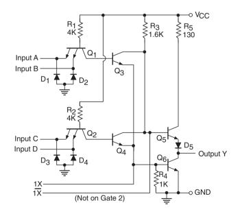
Figure 5.13 Two-input, two-wide AND-OR-INVERT gate.
