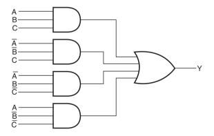
Figure 9.1 Fixed logic circuit.
