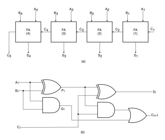
Figure 7.30 Four-bit binary adder.
