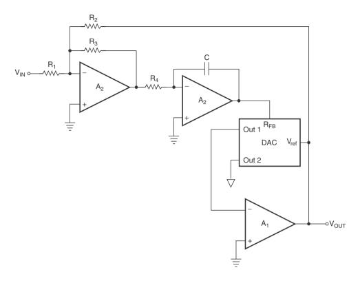
Figure 12.26 Low-pass filter with a programmable time constant.
