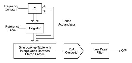
Figure 16.29 Direct digital synthesis.
