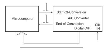
Figure 12.50 A/D converter for data acquisition.
