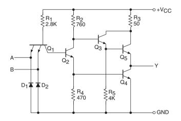
Figure 5.18 NAND gate in the high-power TTL.
