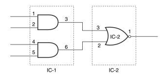
Figure 16.1 Combinational circuit (example 16.1).
