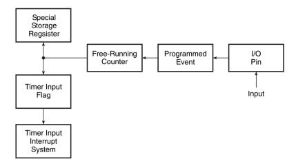
Figure 14.5 Timer input subsystem.
