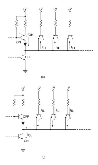
Figure 4.39 Fan-out of the standard TTL logic family.
