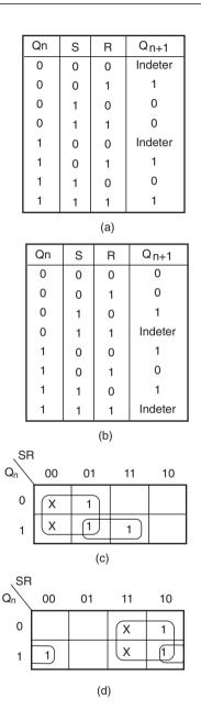
**Figure 10.20** (a) Characteristic table of an *R-S* flip-flop with active LOW inputs, (b) the characteristic table of an *R-S* flip-flop with active HIGH inputs, (c) the K-map solution of an *R-S* flip-flop with active LOW inputs and (d) the K-map solution of an *R-S* flip-flop with active HIGH inputs.
