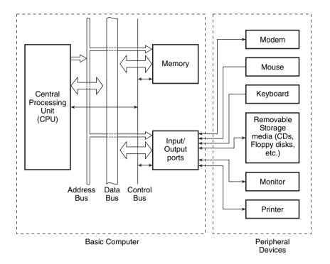
Figure 15.2 Block diagram of a typical computer system.
