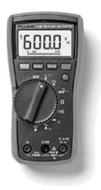
Figure 16.9 Handheld digital multimeter. Reproduced with permission of Fluke Corporation.
