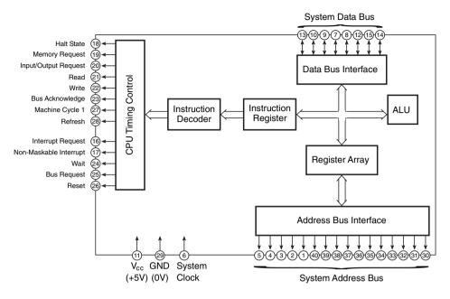
Figure 13.14 Block diagram of Z-80.
