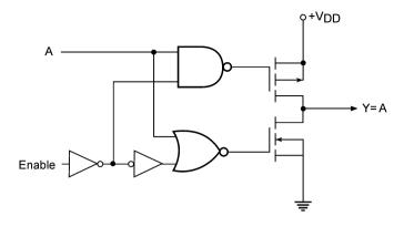
Figure 5.48 Tristate buffer in CMOS.
