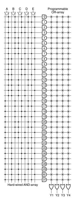
Figure 9.9 Internal architecture of a  $32 \times 4$  PROM.
