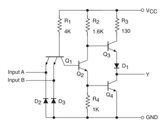
Figure 5.6 Standard TTL NAND gate.
