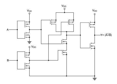
Figure 5.51 Buffered two-input NOR.
