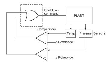
Figure 4.48 Application of an OR gate.
