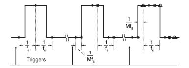
Figure 16.13 Sequential sweep equivalent-time sampling.
