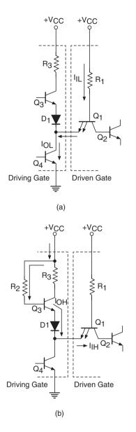
Figure 5.7 (a) Current sinking action and (b) current sourcing action.
