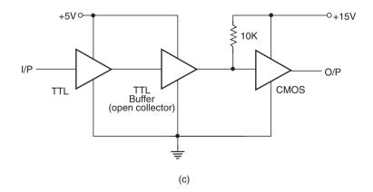
Figure 5.63 TTL-to-CMOS interface.
