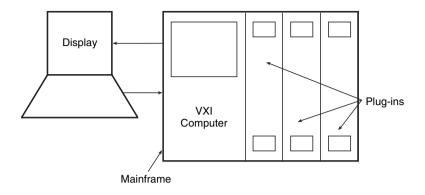
Figure 16.44 VXI-bus computer inside the hardware mainframe.
