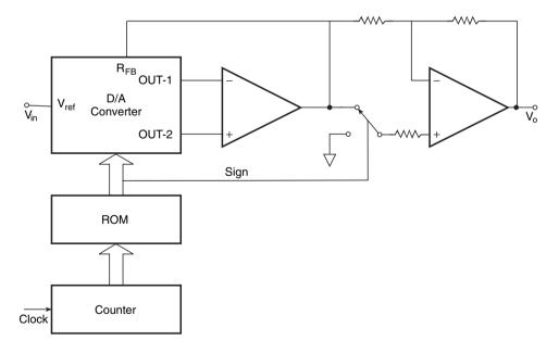
Figure 12.23 Low-frequency function generator.
