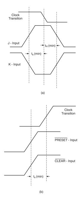
Figure 10.43 Set-up and hold times of a flip-flop.
