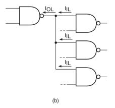
Figure 4.38 Fan-out of logic gates.
