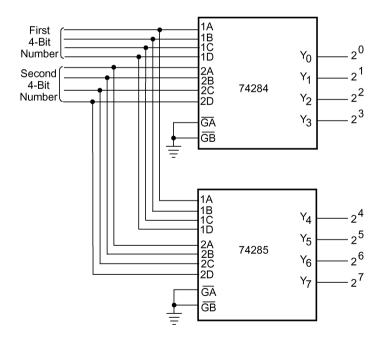
**Figure 7.35**  $4 \times 4$  bit multiplier.
