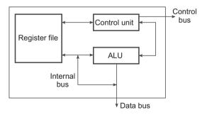
Figure 13.3 Typical schematic arrangement of a microprocessor.
