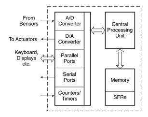
Figure 14.3 Inside the microcontroller.
