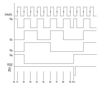
Figure 11.14 Timing waveforms for the counter of Fig. 11.13.
