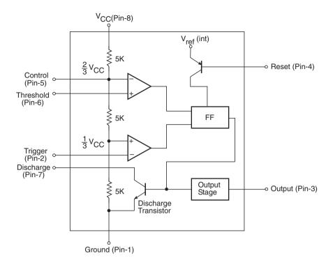
Figure 10.9 Internal schematic of timer IC 555.
