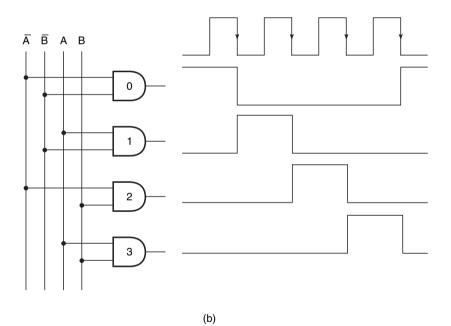
Figure 11.15 MOD-4 ripple counter with decoding logic.
