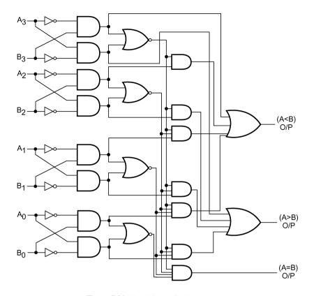
Figure 7.36 Four-bit magnitude comparator.
