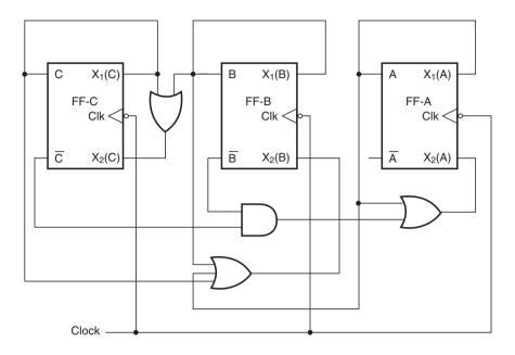
Figure 11.29 Counter circuit (example 11.8).
