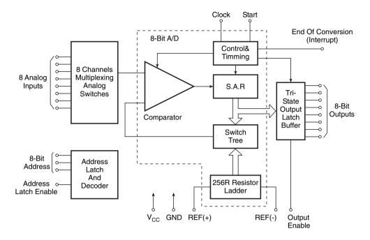
Figure 12.46 Internal architecture/pin connection diagram of AD 7820.
