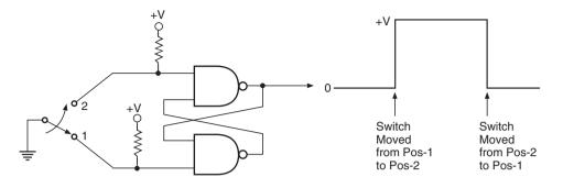
Figure 10.48 Switch debounce circuit.
