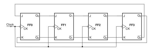
Figure 11.47 Four-bit shift counter.
