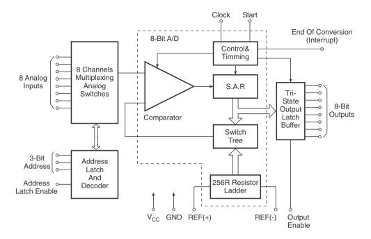
Figure 12.43 Internal architecture of AD 0808.
