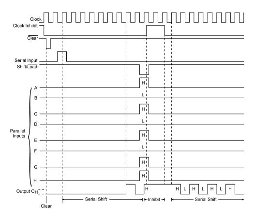
Figure 11.41 Timing waveforms of IC 74166.
