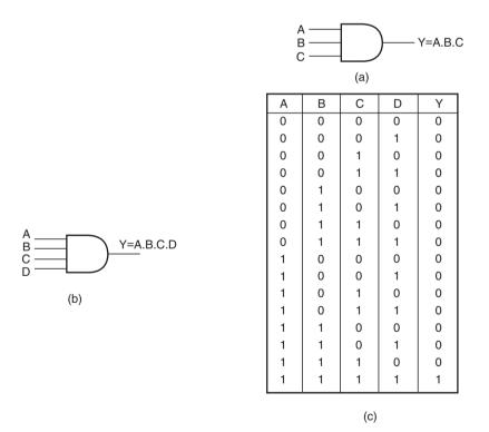
Figure 4.8 (a) Three-input AND gate, (b) four-input AND gate and (c) the truth table of a four-input AND gate.
