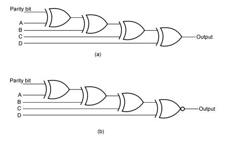
Figure 4.51 Parity check using EX-OR and EX-NOR gates.
