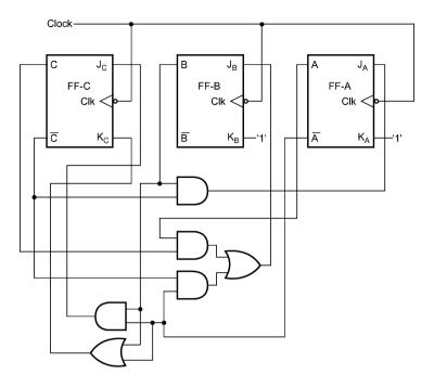
Figure 11.31 Hardware implementation of the counter circuit (example 11.9).
