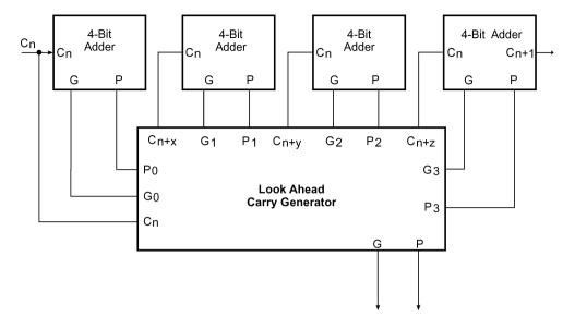
Figure 7.33 IC 74182 interfaced with four four-bit adders.
