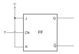
**Figure 10.36** *J*-*K* flip-flop as a *T* flip-flop.
