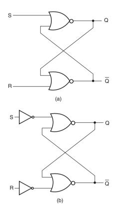
Figure 10.19 NOR implementation of an *R-S* flip-flop.
