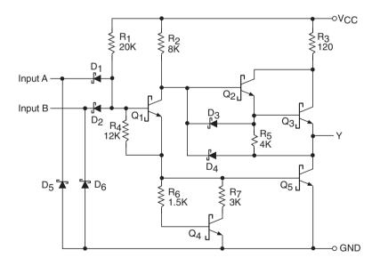
Figure 5.20 NAND gate in the low-power Schottky TTL.
