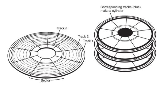
Figure 15.33 Tracks and sectors in a hard disk.
