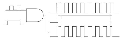
Figure 10.49 Gating of a clock signal.
