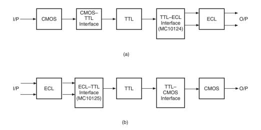
Figure 5.65 CMOS-to-ECL and ECL-to-CMOS interfaces.
