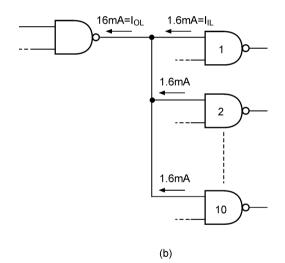
Figure 5.2 Input and output current specifications.
