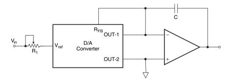
Figure 12.21 Inverting-type programmable integrator.
