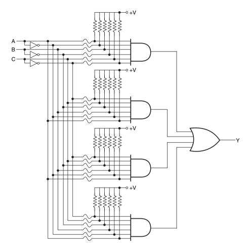
Figure 9.2 Simple programmable logic circuit.
