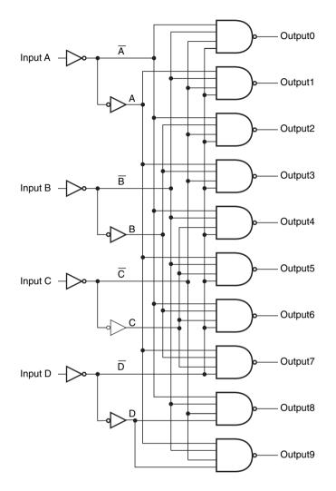
Figure 11.16 Logic diagram of four-line BCD-to-decimal decoder (IC 7442).
