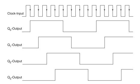
Figure 11.48 Timing waveforms of the shift counter.
