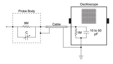
Figure 16.19 Internal circuit of 10X probe.
