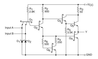
Figure 5.19 NAND gate in the Schottky TTL.
