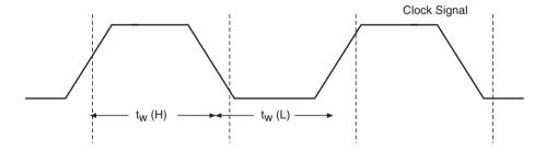
Figure 10.45 Clock pulse HIGH and LOW times.
