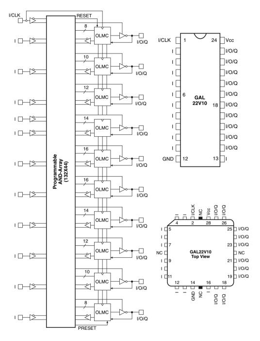
Figure 9.36 Basic architecture and pin connections of 22V10.
