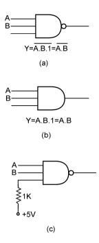
Figure 5.24 Handling unused inputs of AND and NAND gates.
