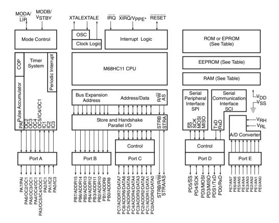
Figure 14.18 Architecture of the 68HC11 family of microcontrollers.
