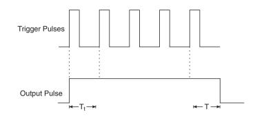
Figure 10.5 Retriggerable monostable multivibrator output for repetitive trigger pulses.
