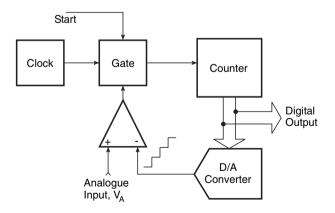
Figure 12.32 Counter-type A/D converter.
