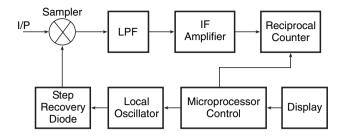
Figure 16.24 Microwave counter architecture.
