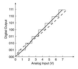
Figure 12.28 Transfer characteristics of a three-bit A/D converter (INL = one LSB, DNL = 1/4 LSB).
