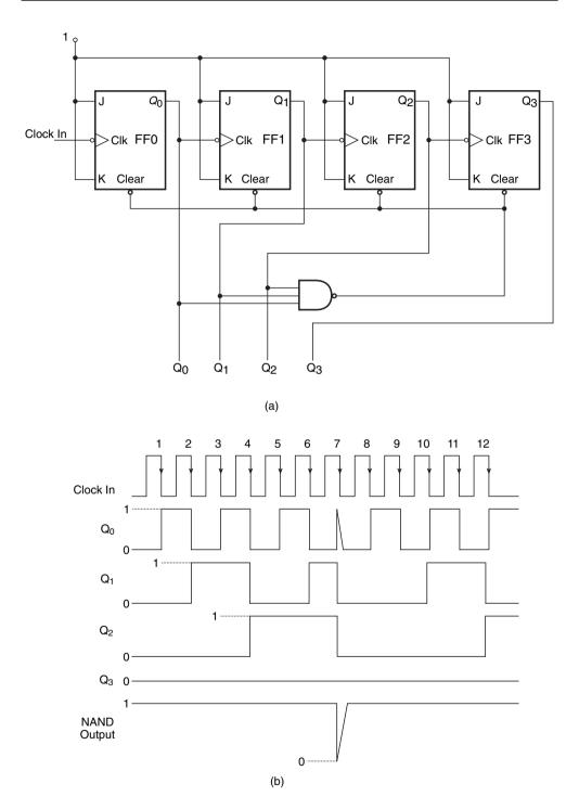
**Figure 11.3** Binary ripple counter with a modulus of less than  $2^N$ .
