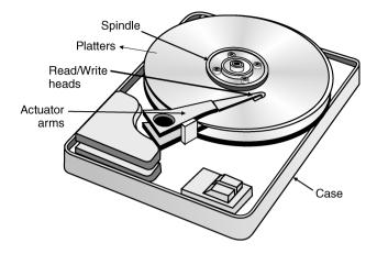
Figure 15.32 Internal structure of a typical hard disk.
