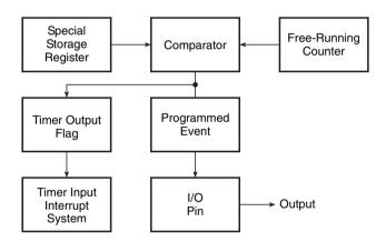
Figure 14.6 Timer output subsystem.
