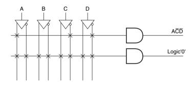
Figure 9.19 Programmability of inputs in a PAL device.
