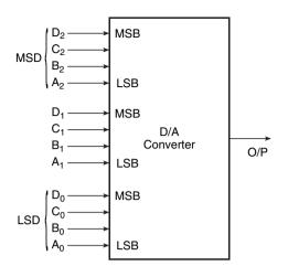
Figure 12.11 BCD-input D/A converter (example 12.2).
