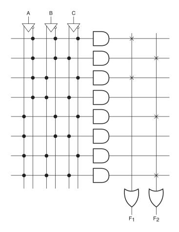
Figure 9.10 8 × 2 PROM internal logic diagram to implement given Boolean function.
