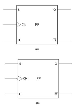
Figure 10.25 (a) Circuit symbol of a positive edge-triggered R-S flip-flop and (b) the circuit symbol of a negative edge-triggered R-S flip-flop.
