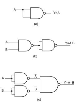
Figure 4.24 Implementation of basic logic gates using only NAND gates.
