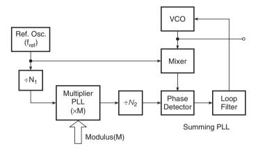
Figure 16.27 Indirect synthesis using more than one PLL.
