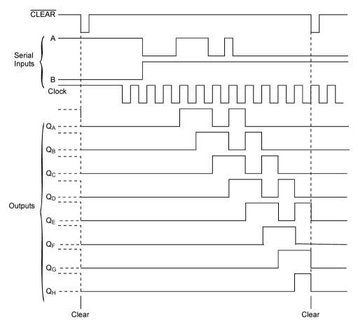
Figure 11.39 Timing waveforms of IC 74164.
