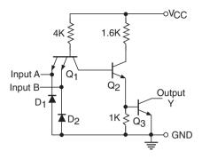
Figure 5.14 NAND gate with an open collector output.
