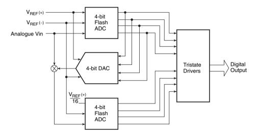
Figure 12.31 Eight-bit half-flash A/D converter.
