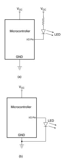
Figure 14.25 Interfacing LEDs to a microcontroller.
