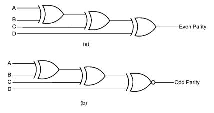
Figure 4.50 Parity generation using EX-OR/EX-NOR gates.
