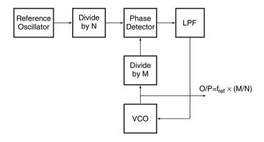
Figure 16.26 Frequency synthesizer architecture – indirect synthesis.
