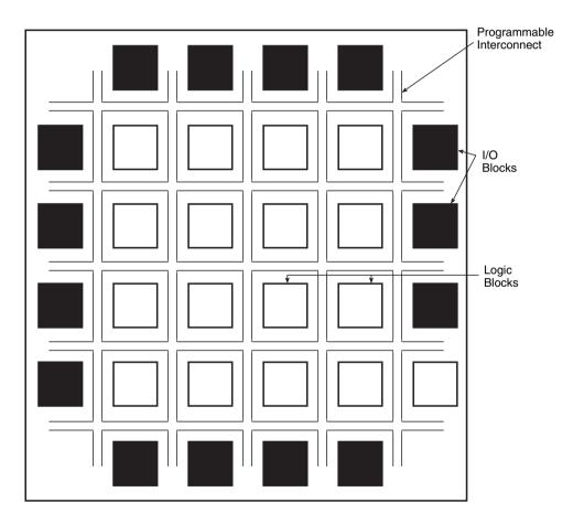
Figure 9.7 FPGA architecture.
