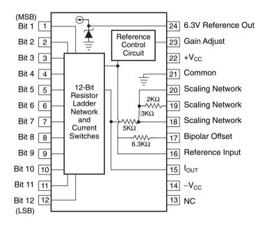
Figure 12.16 Pin connection diagram of DAC-80 (current-output version).
