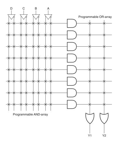
Figure 9.4 Internal architecture of a PLA device.
