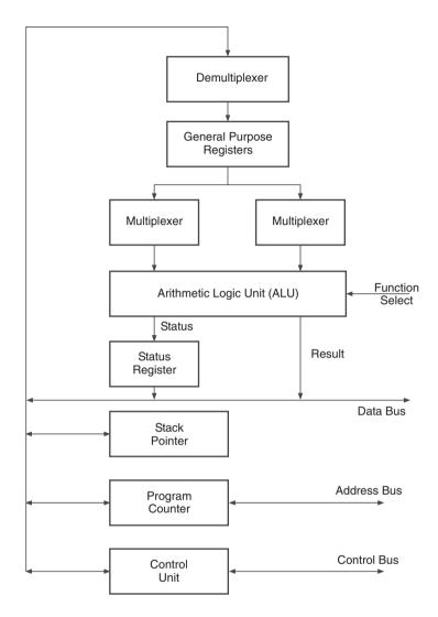
Figure 13.4 Descriptive block diagram of a microprocessor.
