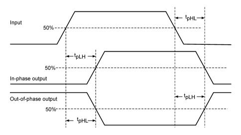
Figure 5.4 Propagation delay parameters.
