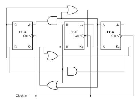
Figure 11.27 Counter with an arbitrary sequence.
