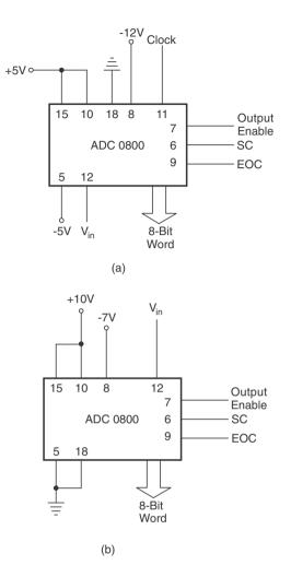
Figure 12.42 Basic application circuits using AD 0800.
