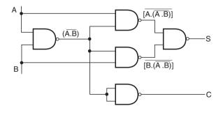
Figure 7.6 Half-adder implementation using NAND gates.
