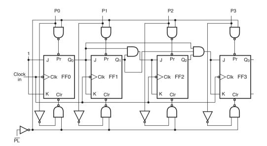
Figure 11.12 Four-bit presettable, clearable counter.
