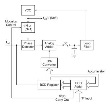
Figure 16.28 Fractional N synthesis.
