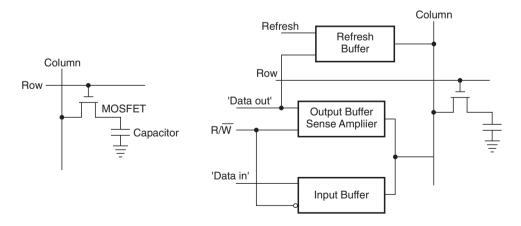
Figure 15.10 Basic memory cell of a DRAM.
