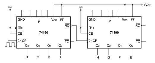
Figure 11.22 Cascade arrangement of two 74190s (example 11.6).
