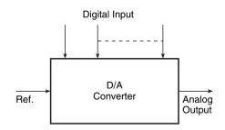
Figure 12.6 Multiplying-type D/A converter.
