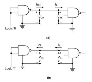
Figure 5.3 (a) HIGH-level current and voltage parameters and (b) LOW-level current and voltage parameters.
