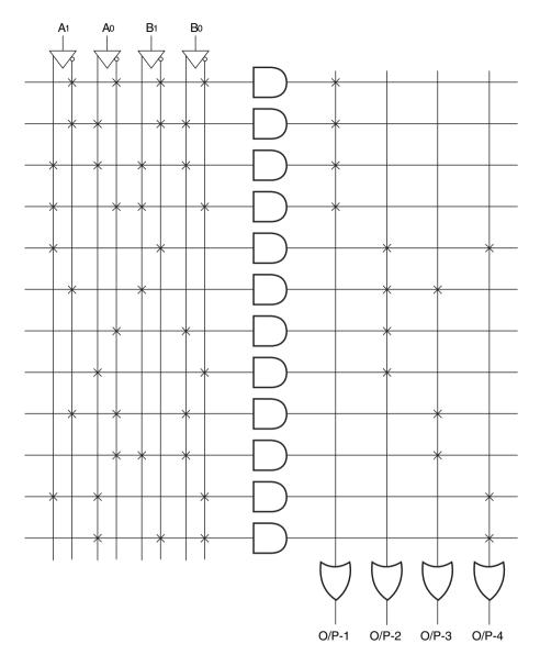
Figure 9.17 Programmed PLA device (example 9.3).
