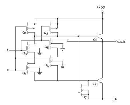
Figure 5.56 BiCMOS two-input NAND.
