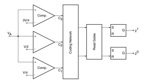
Figure 12.29 Two-bit simultaneous A/D converter.
