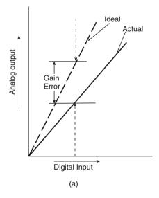
Figure 12.4 (a) Gain error and (b) offset error.
