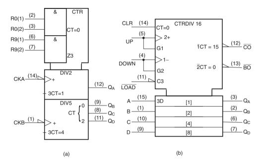
Figure 11.52 IEEE/ANSI notation for (a) IC 7490 and (b) IC 74193.
