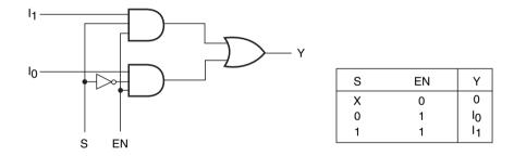
Figure 8.6 2-to-1 multiplexer with an ENABLE input.
