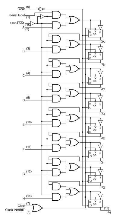
Figure 11.40 Logic diagram of 74166.
