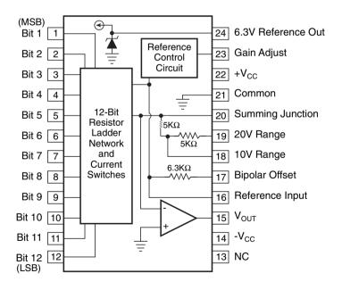
Figure 12.17 Pin connection diagram of DAC-80 (voltage-output version).
