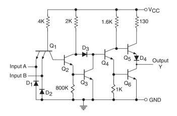
Figure 5.10 AND gate in standard TTL.
