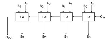
Figure 7.11 Four-bit binary adder.
