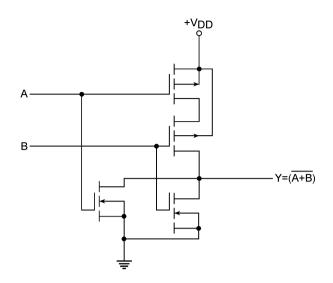
Figure 5.52 Unbuffered two-input NOR.
