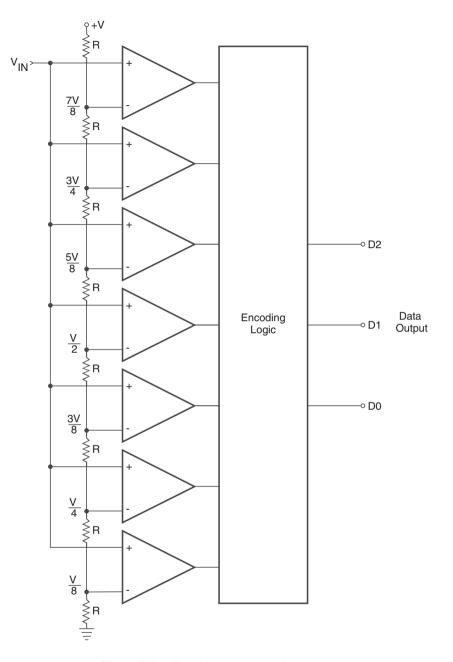
Figure 12.30 Three-bit simultaneous A/D converter.
