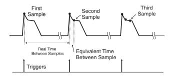
Figure 16.12 Sequential single-sample technique.
