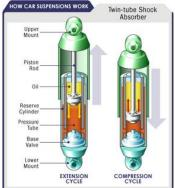
Shocks, or shock absorbers, control unwanted spring motion through a process known as dampening.
