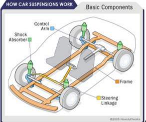
Suspension parts include springs, dampers and
