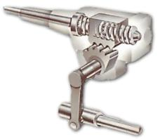
In recirculating-ball steering, the thread between the
