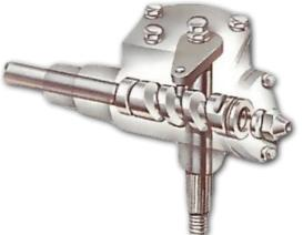
In worm-and-peg steering the worm moves the drop arm by means of a peg connected to a fork.
