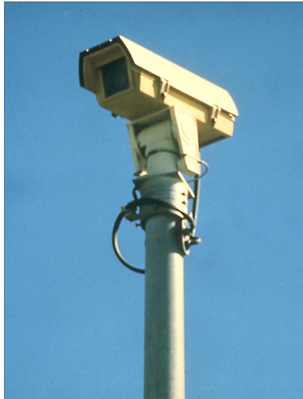
Pan, Tilt and Zoom (PTZ) Closed Circuit TV Camera (Image courtesy of the IBI Group)
