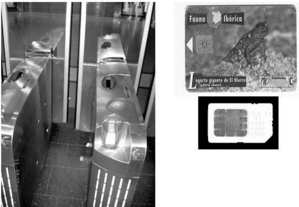
Figure 7.1 Metro electronic ticket reader with smart card reading; a typical example of a smart card; and a smart card for a GSM telephone. (Source: CSI Library.)
